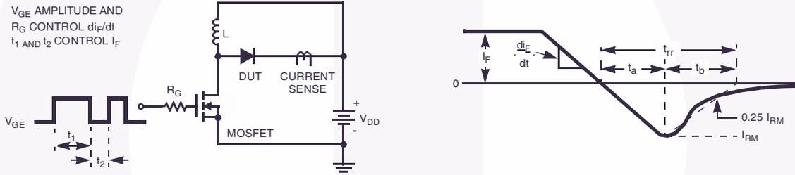
**Figure 1. Diode Reverse Recovery Test Circuit & Waveform**
