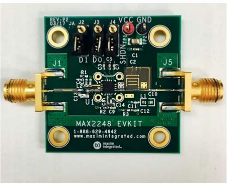
Figure 3. MAX2248 EV kit tuned for 2.4GHz.
