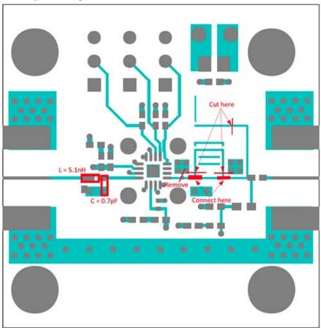
Figure 2. MAX2248 EV kit PCB changes for 2.4GHz tuning.
