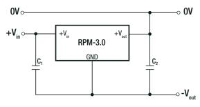
${\bf C_1}$  and  ${\bf C_2}$  may be added to reduced ripple and should be fitted close to the converter pins.
