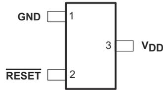
**Figure 6-1. Pin configuration**
