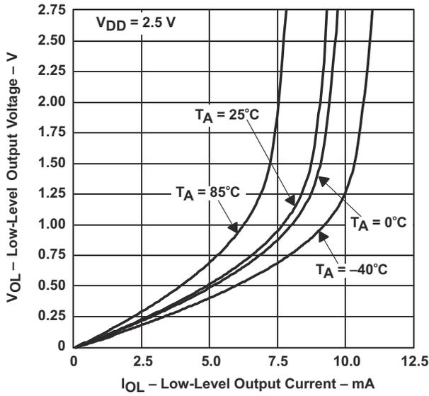
Figure 7-1. LOW-LEVEL OUTPUT VOLTAGE vs LOW-LEVEL OUTPUT CURRENT
