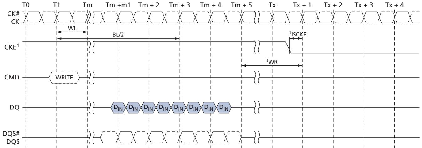
Note: 1. CKE can be registered LOW at  $(WL + 1 + BL/2 + RU(tWR/tCK))$  clock cycles after the clock on which the WRITE command is registered.
