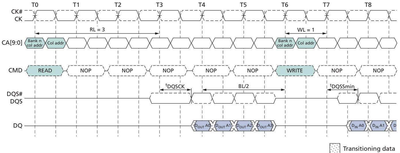
The minimum time from the burst READ command to the burst WRITE command is defined by the read latency (RL) and the burst length (BL). Minimum READ-to-WRITE latency is  $RL + RU(t_{DQSCK}(MAX)/t_{CK}) + BL/2 + 1 - WL$  clock cycles. Note that if a READ burst is truncated with a burst TERMINATE (BST) command, the effective burst length of the truncated READ burst should be used for BL when calculating the minimum READ-to-WRITE delay.
