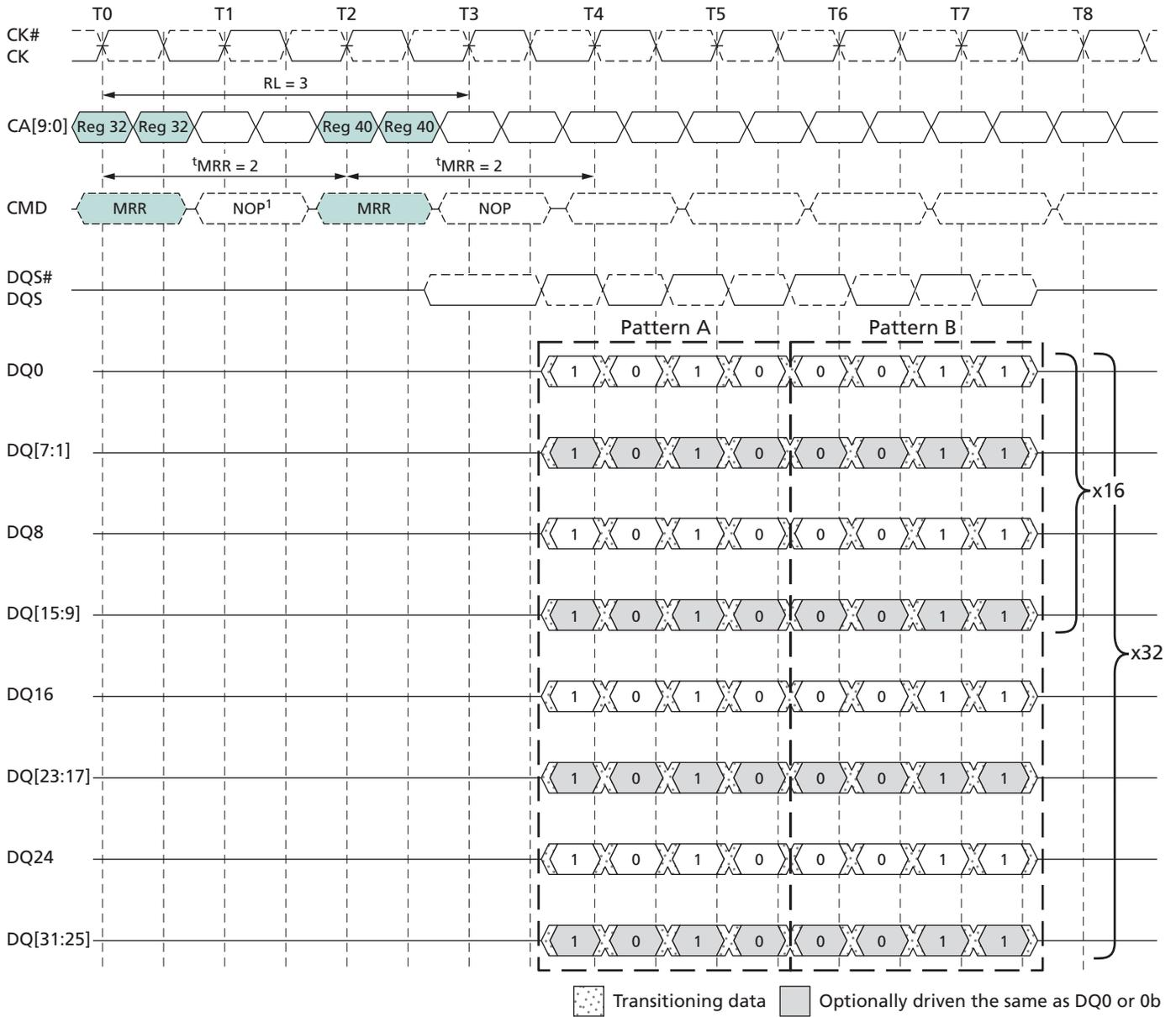
Note: 1. Only the NOP command is supported during  $t_{MRR}$ .
