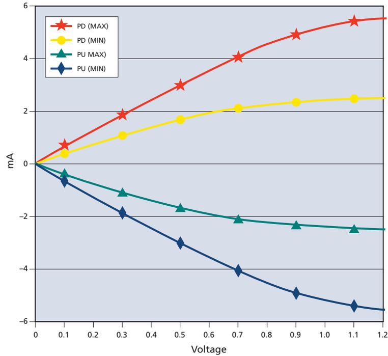
Figure 79: Output Impedance = 240 Ohms, I-V Curves After Calibration
