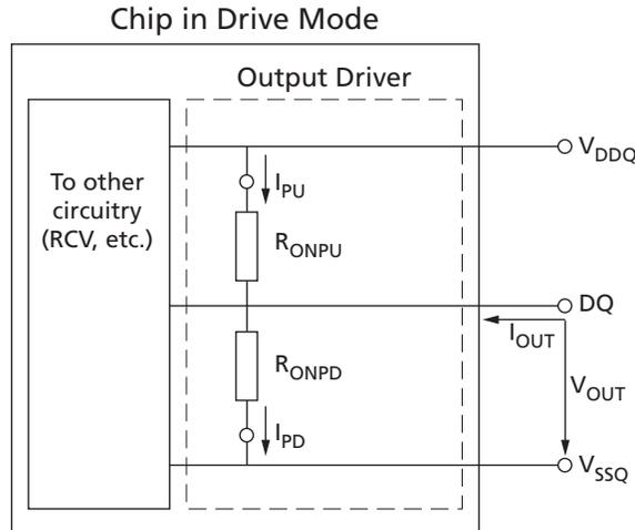
**Output Driver Impedance Characteristics with ZQ Calibration**
