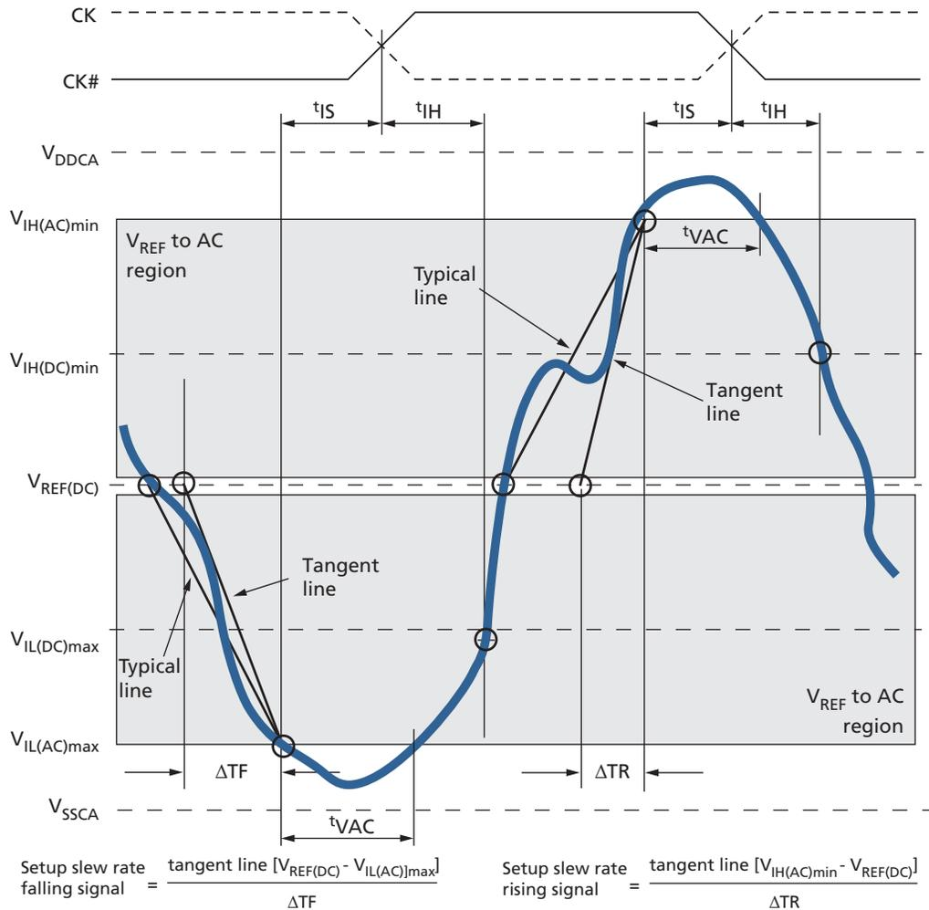
**Figure 84: Tangent Line –  $t_{IH}$  for CA and CS# Relative to Clock**
