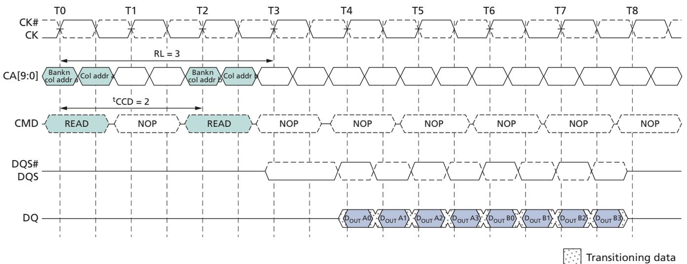
A seamless burst READ operation is supported by enabling a READ command at every other clock cycle for BL = 4 operation, every fourth clock cycle for BL = 8 operation, and
