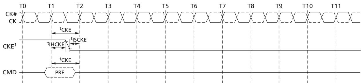
Note: 1. CKE can go LOW  $t_{IHCKE}$  after the clock on which the PRECHARGE command is registered.
