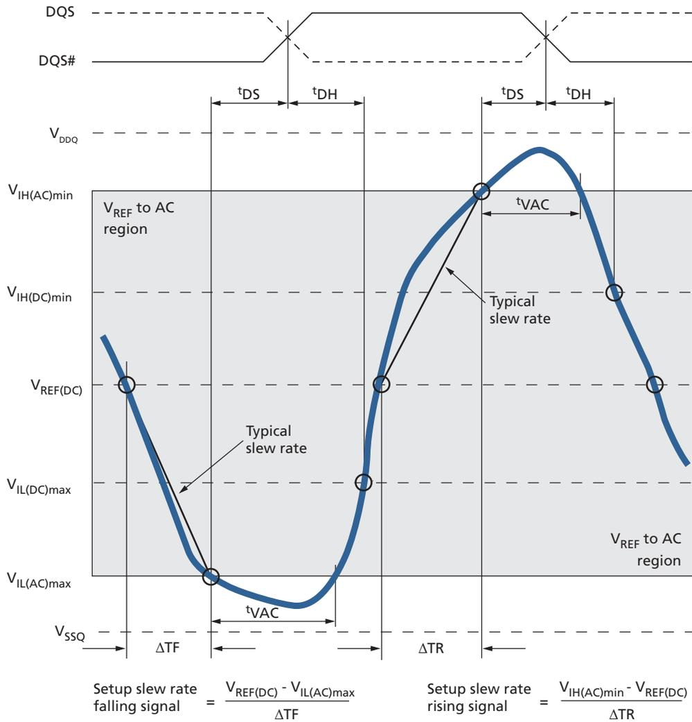
**Figure 86: Typical Slew Rate – t<sub>DH</sub> for DQ Relative to Strobe**
