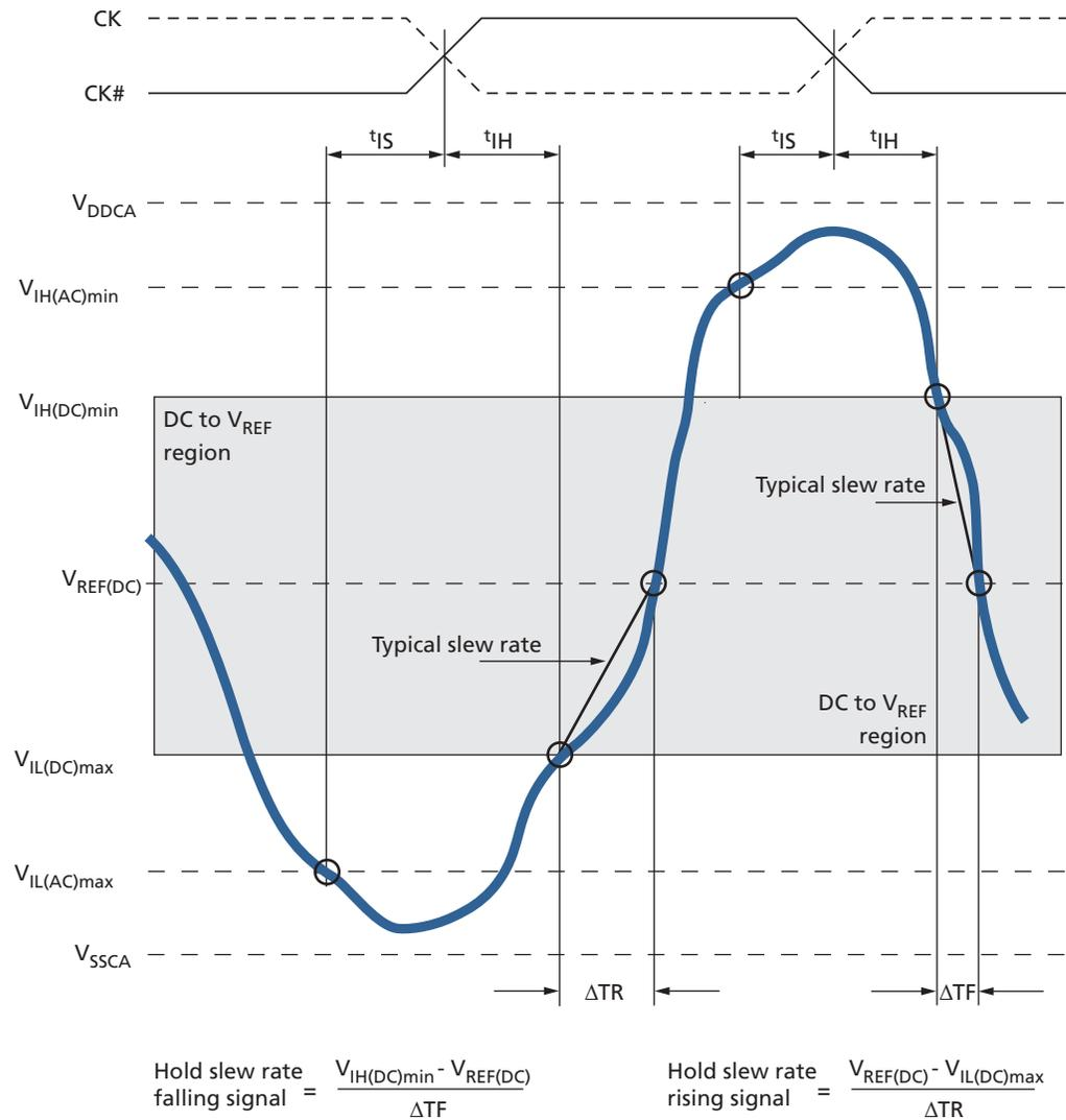
Figure 83: Tangent Line –  $t_{IS}$  for CA and CS# Relative to Clock
