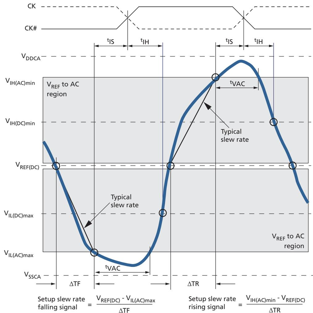
**Figure 82: Typical Slew Rate –  $t_{IH}$  for CA and CS# Relative to Clock**
