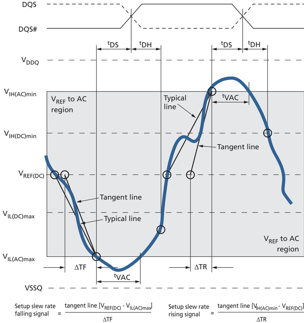
**Figure 88: Tangent Line – t<sub>DH</sub> for DQ with Respect to Strobe**
