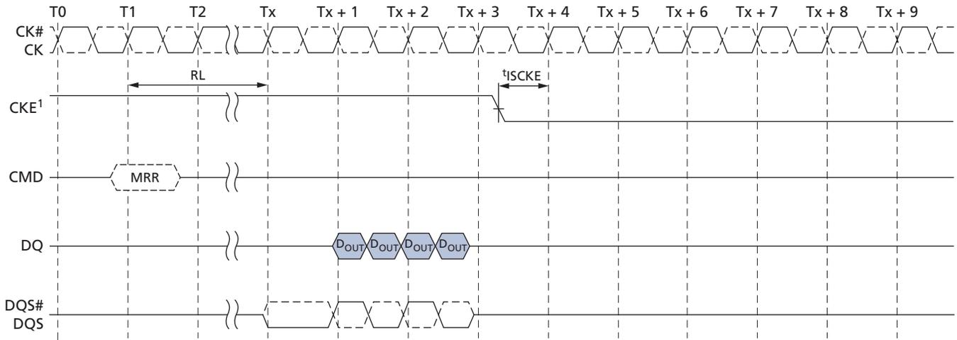
Note: 1. CKE can be registered LOW at  $(RL + RU(t_{DQ\text{SCK}}/t_{CK}) + BL/2 + 1)$  clock cycles after the clock on which the MRR command is registered.
