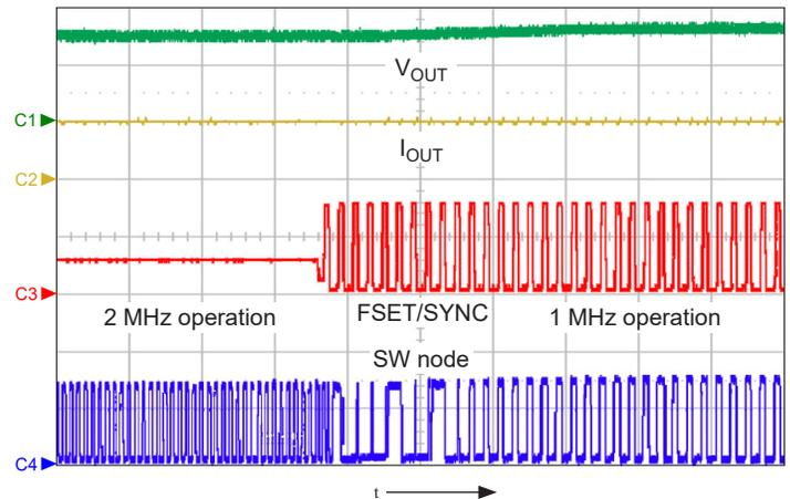
Figure 9: Transition of the SW waveform when the SYNC pulse is detected. The A8514 switching at 2 MHz, applied SYNC pulse at 1 MHz; shows  $V_{OUT}$  (ch1, 20 V/div.),  $I_{OUT}$  (ch2, 200 mA/div.), FSET/SYNC (ch3, 2 V/div.), and SW node (ch4, 20 V/div.), time = 5  $\mu$ s/div.
