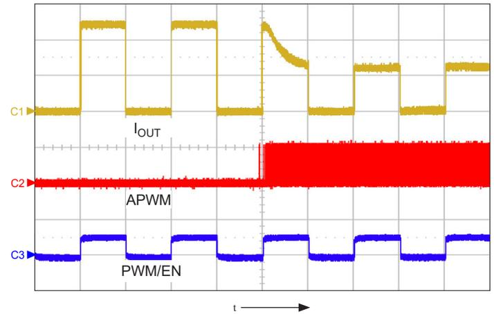
Figure 21: Transition of output current level when a 50% duty cycle signal is applied to the APWM pin, in conjunction with a 50% duty cycle PWM dimming being applied to the PWM pin; shows  $I_{OUT}$  (ch1, 50 mA/div.), APWM (ch2, 10 V/div.), and PWM/EN (ch3, 5 V/div.), time = 500  $\mu$ s/div.
