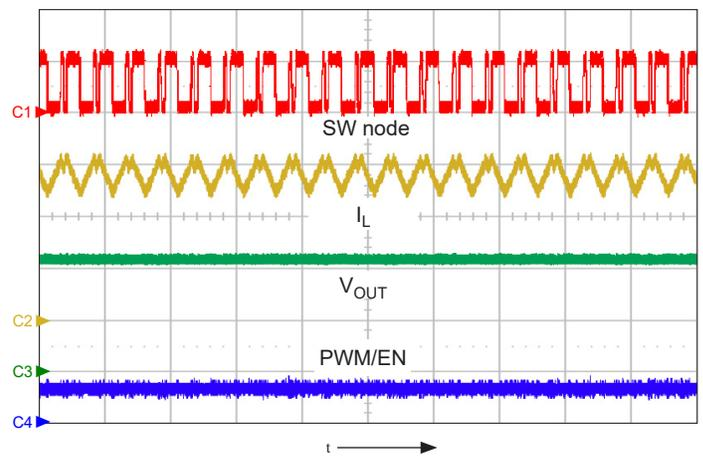
Figure 29: Cycle-by-cycle current limiting; inductor current (yellow trace,  $I_L$ ), note reduction in output voltage as compared to normal operation with the same configuration (Figure 27); shows SW node (ch1, 20 V/div.), inductor current  $I_L$  (ch2, 1 A/div.),  $V_{OUT}$  (ch3, 10 V/div.), and PWM/EN (ch4, 5 V/div.), time = 2  $\mu$ s/div.
