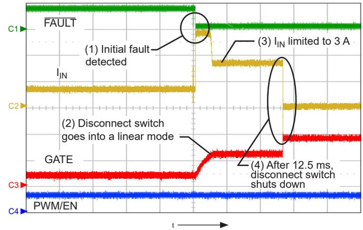
Figure 32: Showing typical wave forms for a 3-A, 1X current limit under a fault condition; shows  $f_{SW} = 800$  kHz, FAULT (ch1, 5 V/div.),  $I_{IN}$  (ch2, 2 A/div.), GATE (ch3, 5 V/div.), and PWM/EN (ch4, 5 V/div.), time = 5 ms/div.
