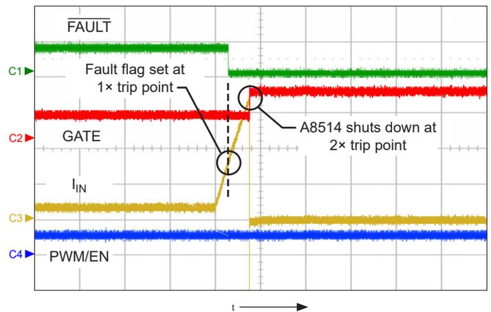
Figure 33: 2x mode, secondary overcurrent fault condition.  $I_{IN}$  is the input current through the switch. The Fault flag is set at the 1x current limit, and when the 2x current limit is reached the A8514 disables the gate of the disconnect switch (GATE); shows FAULT (ch1, 5 V/div.), GATE (ch2, 10 V/div.),  $I_{IN}$  (ch3, 2 A/div.), and PWM/EN (ch4, 5 V/div.), time = 5  $\mu$ s/div.
