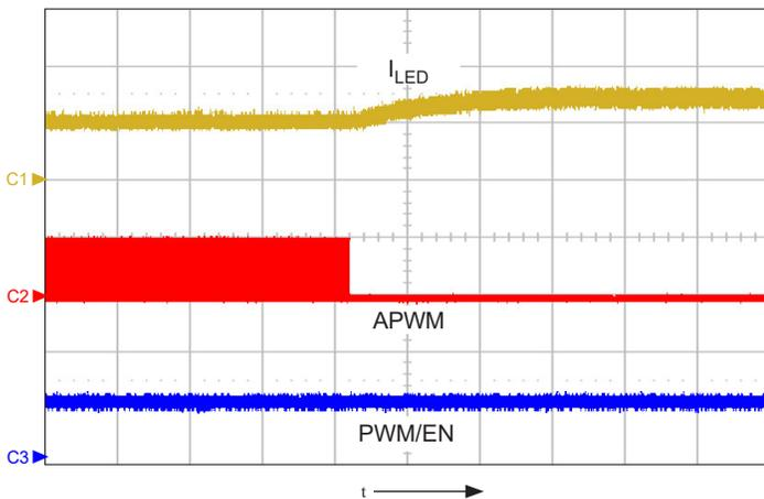
Figure 18: Diagram showing the transition of LED current from 60 mA to 80 mA, when a 25% duty cycle signal is removed from the APWM pin. PWM = 1; shows  $I_{LED}$  (ch1, 50 mA/div.), APWM (ch2, 10 V/div.), and PWM/EN (ch3, 5 V/div.), time = 500  $\mu$ s/div.
