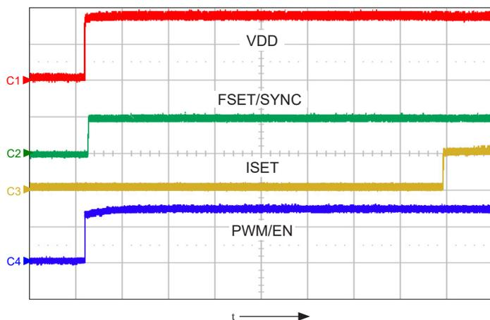
Figure 3: Power-up diagram; shows VDD (ch1, 2 V/div.), FSET/SYNC (ch2, 1 V/div.), ISET (ch3, 1 V/div.), and PWM/EN (ch4, 2 V/div.) pins, time = 200  $\mu$ s/div.
