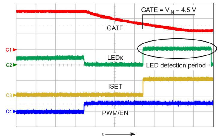
Figure 2: Power-up diagram; shows the relationship of an LEDx pin with respect to the gate voltage of the disconnect switch (if used) during the LED detect phase, as well as the duration of the LED detect phase for a switching frequency of 2 MHz; shows GATE (ch1, 5 V/div.), LED (ch2, 500 mV/div.), ISET (ch3, 1 V/div.), and PWM/EN (ch4, 5 V/div.) pins, time = 500  $\mu$ s/div.
