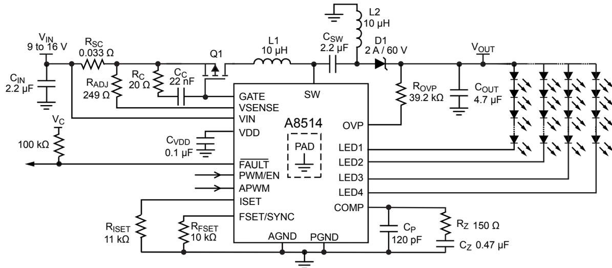
Figure 37: Typical application showing SEPIC configuration, with accurate input current sense, and VSENSE to ground protection.
