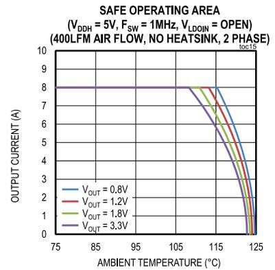
( $V_{DDH} = 12V$ , tested on MAX20808EVKIT#,  $T_A = +25^\circ C$ , unless otherwise noted.)
