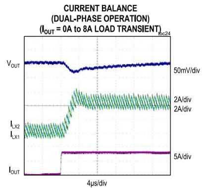
( $V_{DDH} = 12V$ , tested on MAX20808EVKIT#,  $T_A = +25^\circ C$ , unless otherwise noted.)
