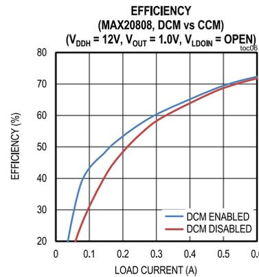
( $V_{DDH} = 12V$ , tested on MAX20808EVKIT#,  $T_A = +25^\circ C$ , unless otherwise noted.)
