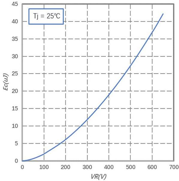
Fig.5-Capacitance Stored Energy
