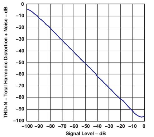
Figure 15. Total Harmonic Distortion + Noise vs Signal Level
