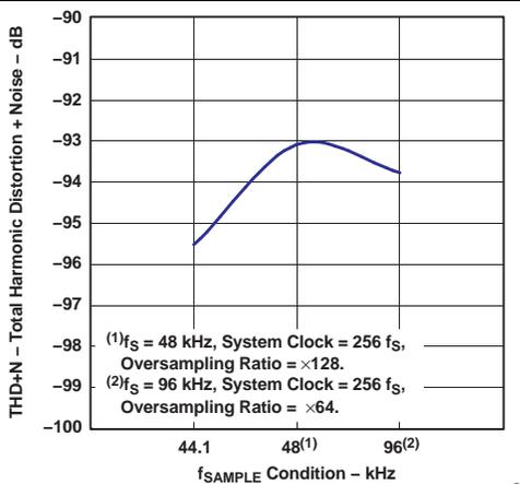
Figure 11. Total Harmonic Distortion + Noise vs  $f_{\text{SAMPLE}}$  Condition
