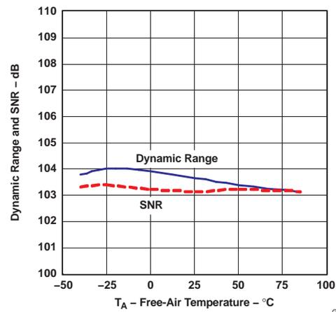
Figure 8. Dynamic Range and Signal-to-Noise Ratio vs Temperature
