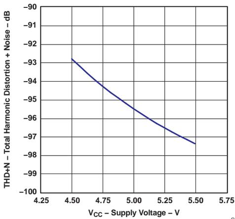
Figure 9. Total Harmonic Distortion + Noise vs Supply Voltage
