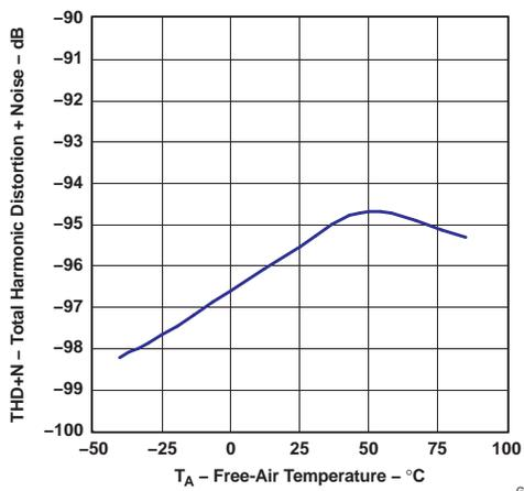
Figure 7. Total Harmonic Distortion + Noise vs Temperature
