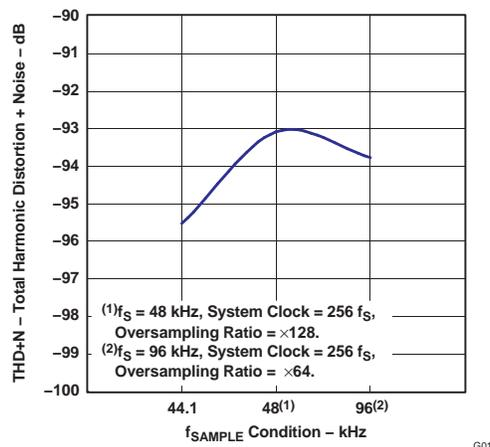
**Figure 25. Total Harmonic Distortion + Noise vs f<sub>SAMPLE</sub> Condition**
