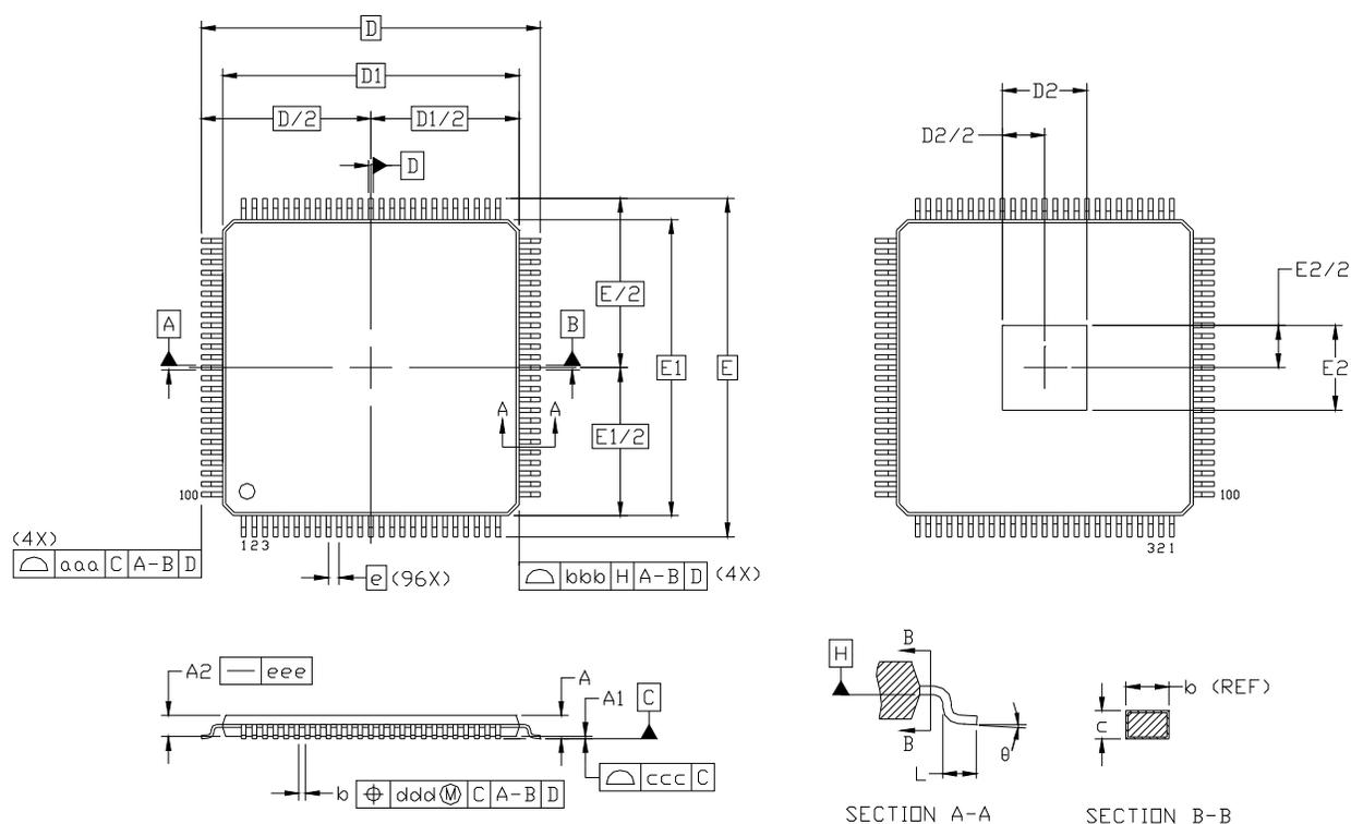
**Figure 9. 100-Pin Thin Quad Flat Package (TQFP)**
