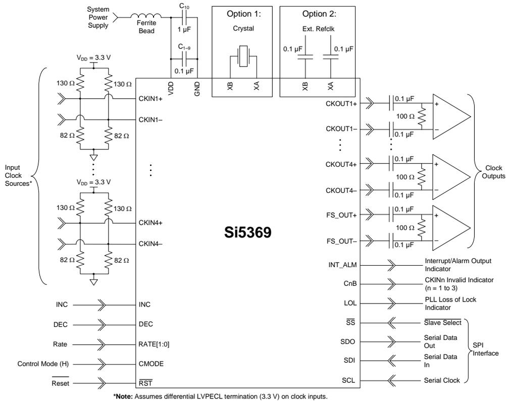
**Figure 8. Si5369 Typical Application Circuit (SPI Control Mode)**
