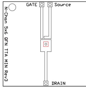
Max  $R_{\theta JA} = 125^{\circ}\text{C/W}$
