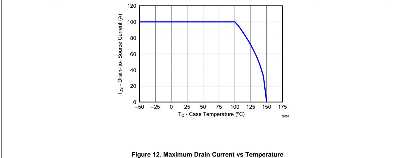
Figure 12. Maximum Drain Current vs Temperature
