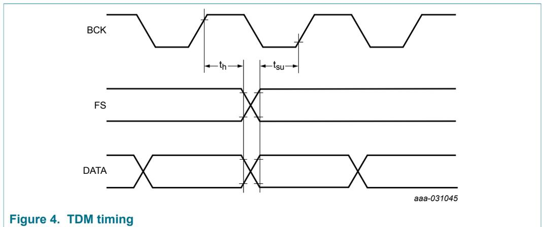
Figure 4. TDM timing
