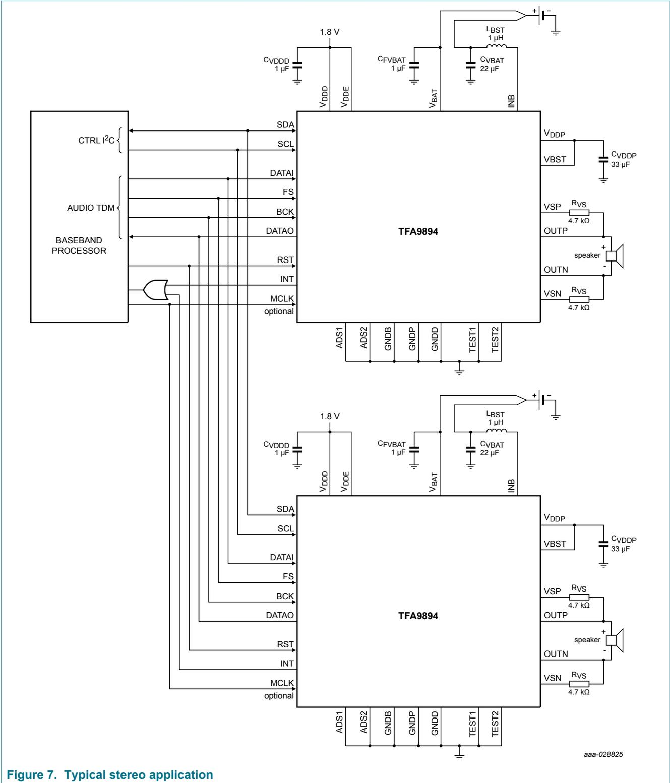
Figure 7. Typical stereo application
