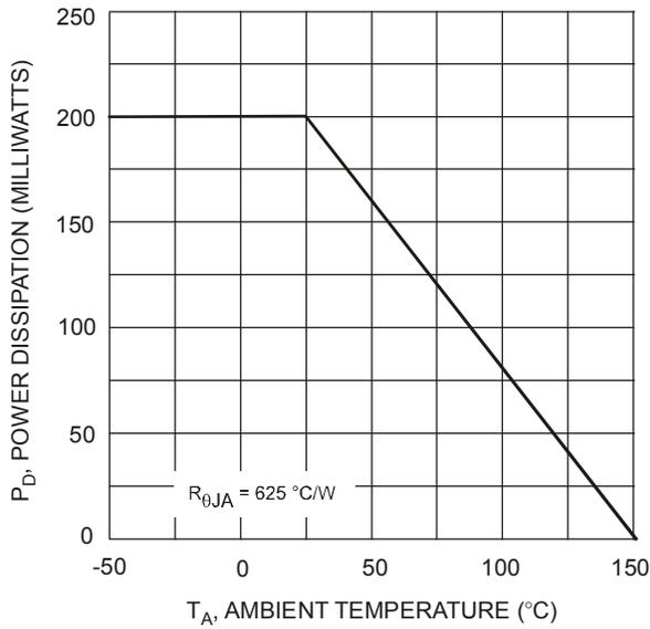
Fig. 1 Derating Curve
