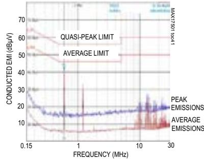
Measured on the MAX17501FTEVKIT with input filter—
