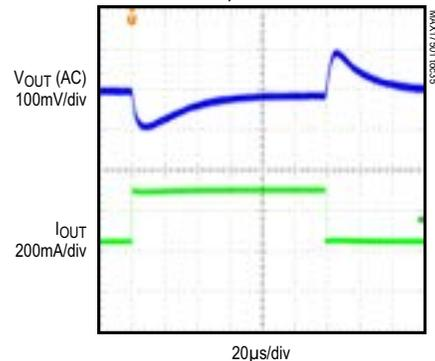
SWITCHING WAVEFORMS OF MAX17501F
