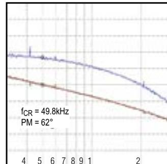
MAX17501, 5V OUTPUT, 0.5A LOAD CURRENT, FIGURE 7 CIRCUIT, CONDUCTED EMI CURVE
