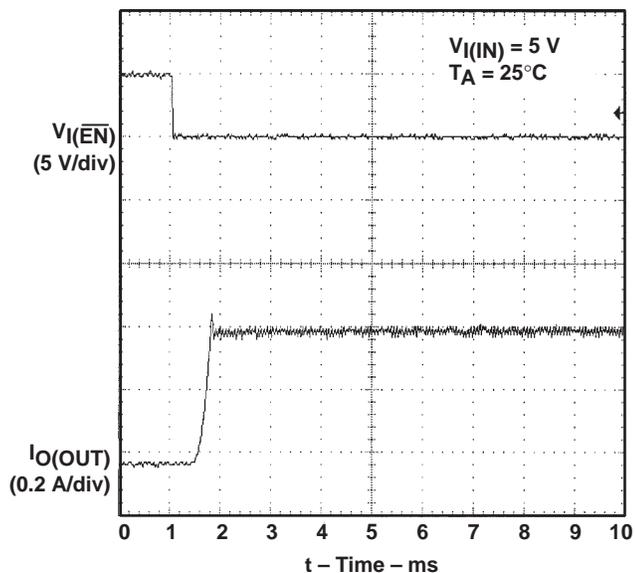
Figure 6. TPS2045, Short-Circuit Current, Device Enabled into Short
