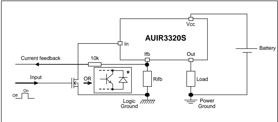
\*The diode between the collector and the emitter is necessary for the reverse battery protection
