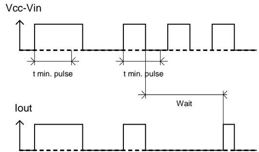
**Figure 3 – Active clamp waveforms**
