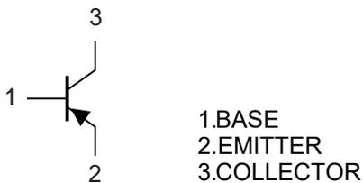
**PNP Silicon Plastic-Encapsulate Transistor**
