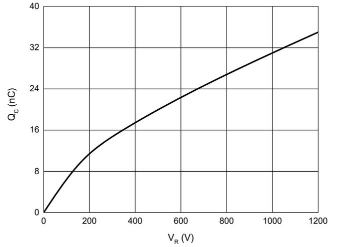
Fig. 5 - Capacitance Stored Energy
