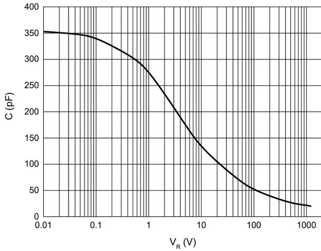
Fig. 4 - Capacitive Charge vs Reverse Voltage
