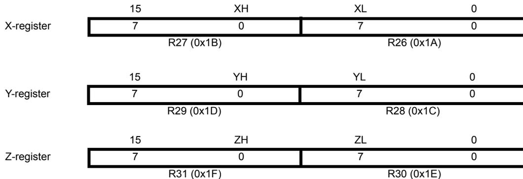
In the different addressing modes these address registers have functions as fixed displacement, automatic increment, and automatic decrement (see Section 30. "Instruction Set Summary" on page 312).
