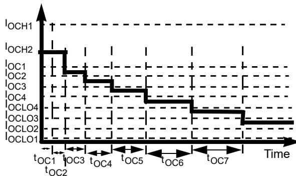
**Figure 18. Overcurrent profile with OCHI bit set to '1'**
