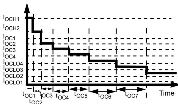
**Figure 17. Overcurrent profile depending on  $\overline{\text{Xenon}}$  bit**
