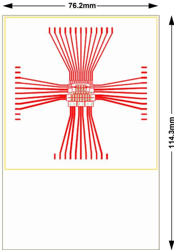
**Figure 22. 2s2p JDEC thermal test board**
