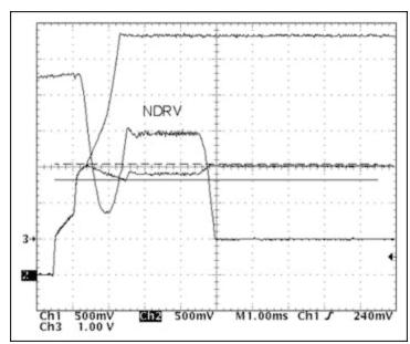
Figure 9. Startup waveforms without lead network.
