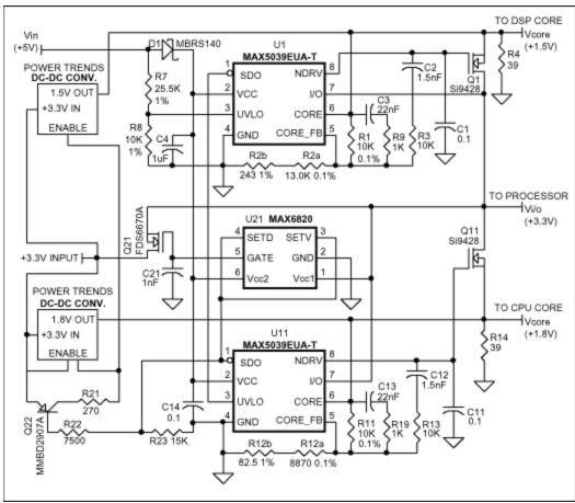
Figure 22. Complete parallel type-B system circuit.
