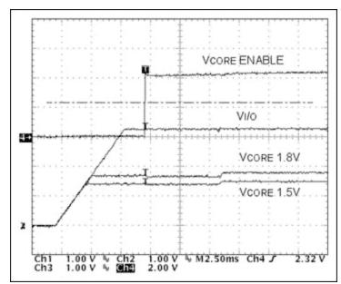
Figure 11. Dual tracking startup waveforms.
