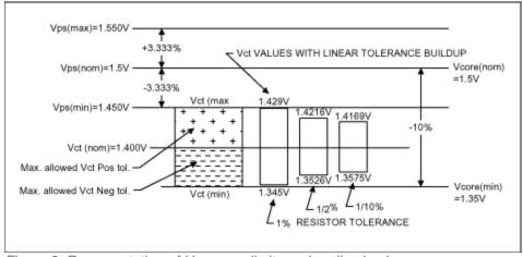
Figure 6. Representation of V<sub>CT</sub> error limits and realized values.
