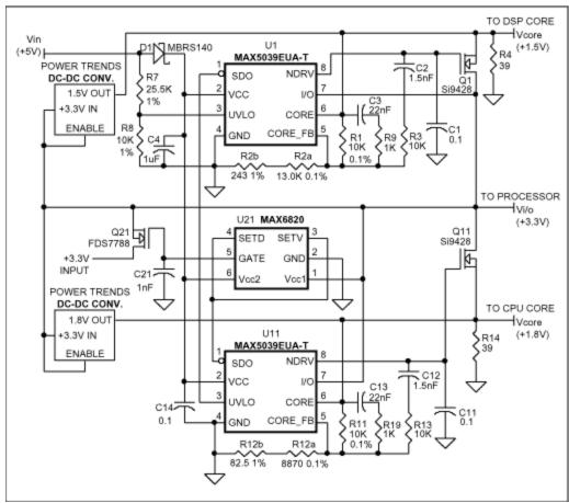
Figure 21. Complete cascade type-B system circuit.
