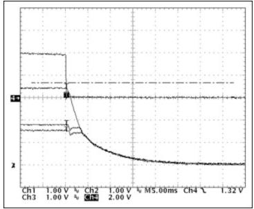
Figure 12. Dual tracking shutdown waveforms.
