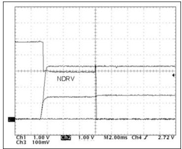
Figure 10. Startup waveforms with lead network.
