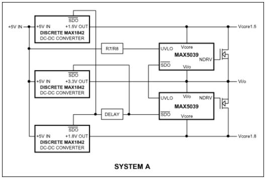
Figure 15. Parallel type-A system with discrete converters.
