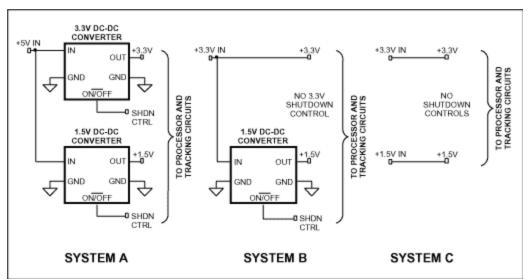
Figure 13. Three basic power system source configurations.
