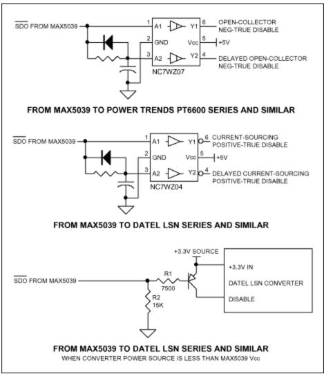
Figure 19. Enable signal interface ciruit options including delayed options.
