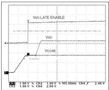
Figure 5. Startup operation, V<sub>CORE</sub> enable preceeds V<sub>I/O</sub> enable.
