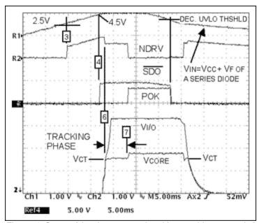
Figure 4. Startup/shutdown operation,  $V_{I/O}$  enable preceeds  $V_{CORE}$  enable.
