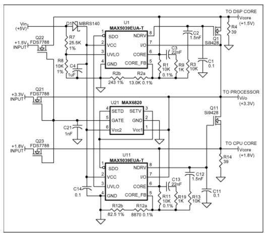
Figure 23. Complete type-C system circuit.
