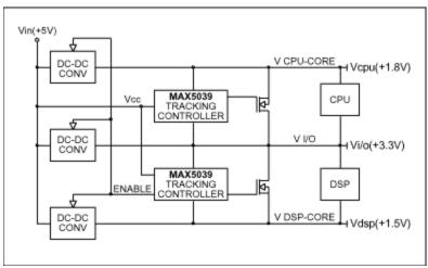
Figure 1. Basic dual voltage-tracking control.
