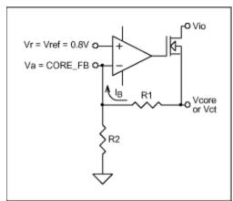
Figure 7. Tracking-voltage control loop.
