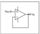
Figure 8. Reference voltage measurement circuit.
