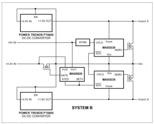
Figure 16. Cascade type-B system.
