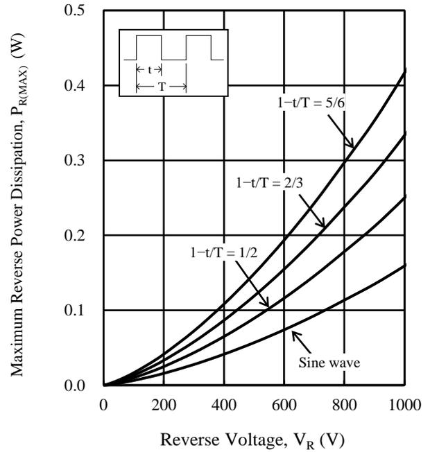
Figure 5.  $P_{R(MAX)}$  vs.  $V_R$  ( $T_J = 150\text{ }^\circ\text{C}$ )
