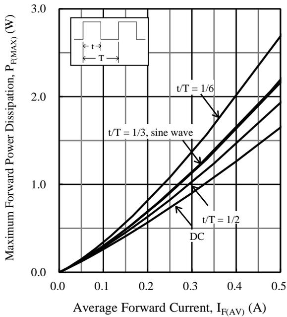
Figure 4.  $P_{F(MAX)}$  vs.  $I_{F(AV)}$  ( $T_J = 150\text{ }^\circ\text{C}$ )
