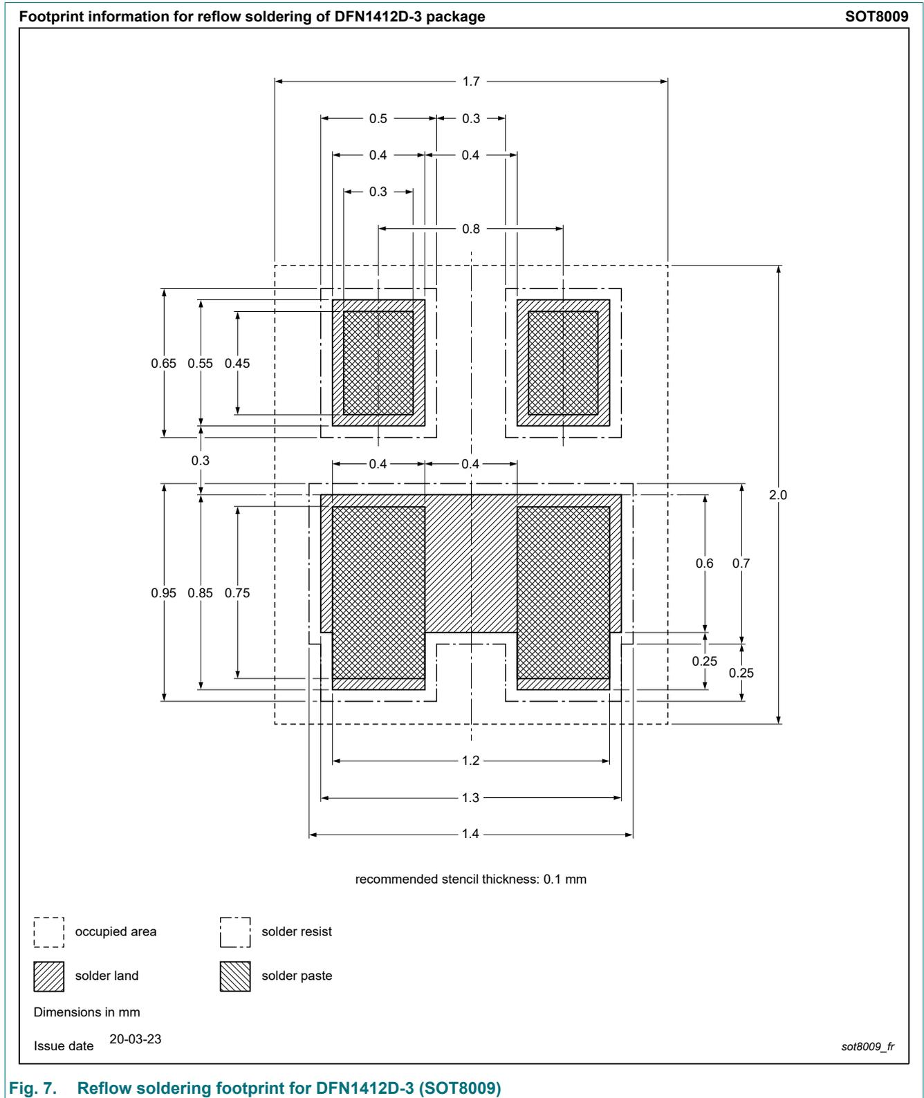
**Fig. 7. Reflow soldering footprint for DFN1412D-3 (SOT8009)**
