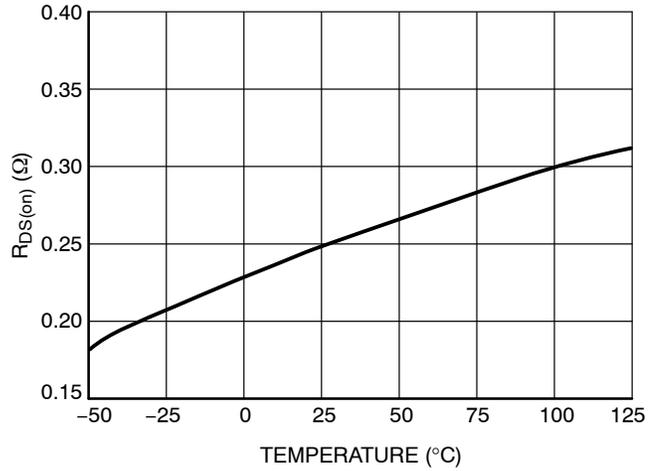
Figure 8. R<sub>DS(on)</sub> vs. Temperature
