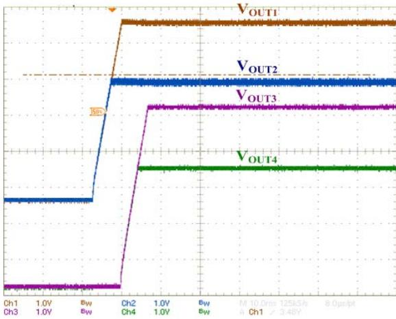
Figure 66. Mixed Mode of Four Outputs – Power-up
