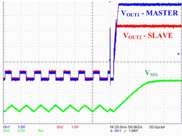
Figure 62. Master Voltage – End of OLM
