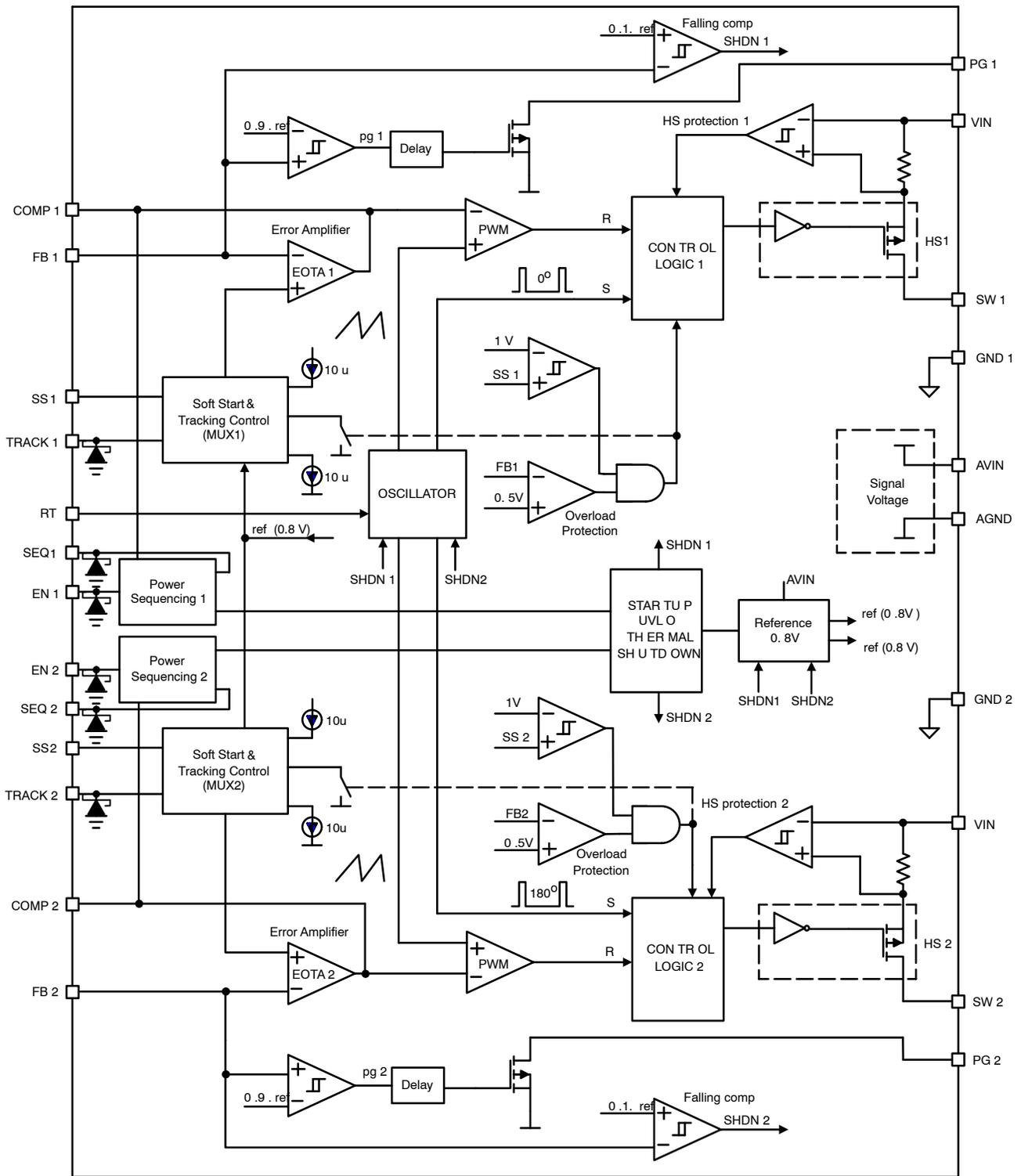
Figure 2. Block Diagram
