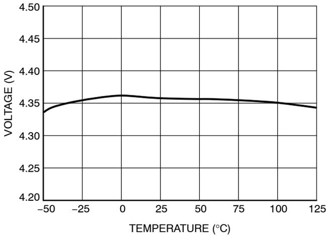
Figure 9. UVLO - Rising Threshold vs. Temperature
