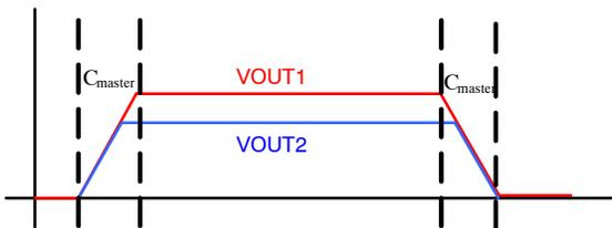
Figure 54. Tracking Configuration
