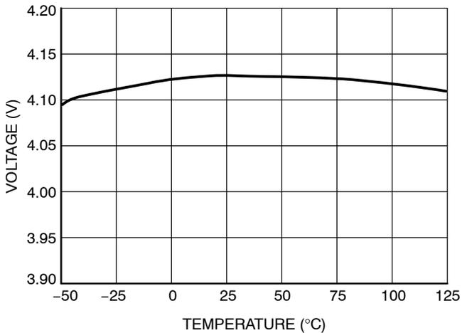
Figure 11. UVLO - Falling Threshold vs. Temperature
