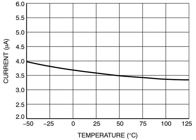
Figure 20. EN Internal Pull-up Current vs. Temperature
