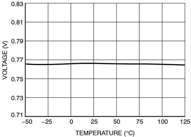
Figure 17. Power Good Feedback Threshold vs. Temperature
