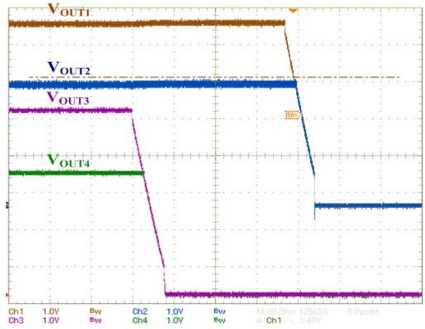
Figure 67. Mixed Mode of Four Outputs – Power-down
