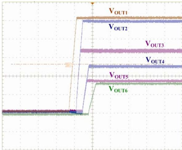
Figure 69. Mixed Mode of Six Outputs – Power-up
