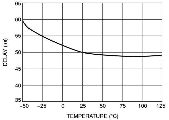
Figure 16. Power Good Rising Delay vs. Temperature
