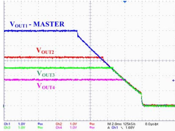
Figure 59. Tracking Mode of Four Outputs – Power-down
