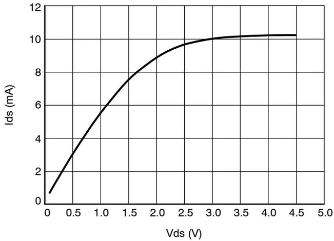
Figure 21. Power Good Current vs. Drain-to-Source Voltage
