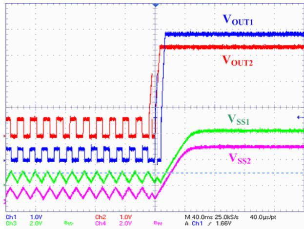
Figure 45. Ratiometric Mode – End of OLM
