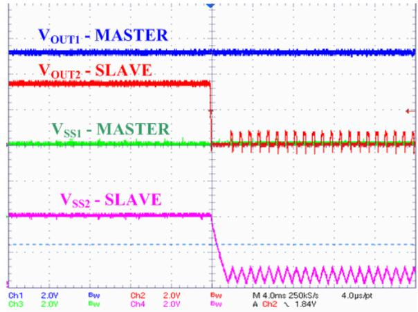
Figure 64. Master Voltage – End of Augmented OLM
