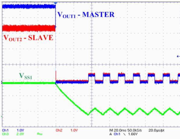
Figure 61. Master Voltage – Start of OLM
