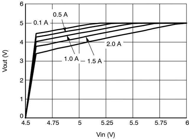
Figure 33. Minimum Input Voltage 5 Vout, 350 kHz
