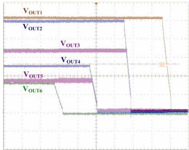
Figure 70. Mixed Mode of Six Outputs – Power-down
