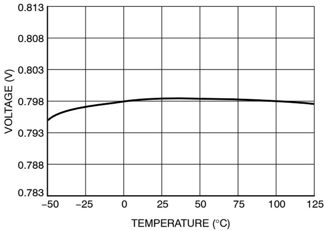
Figure 3. Feedback Voltage vs. Temperature
