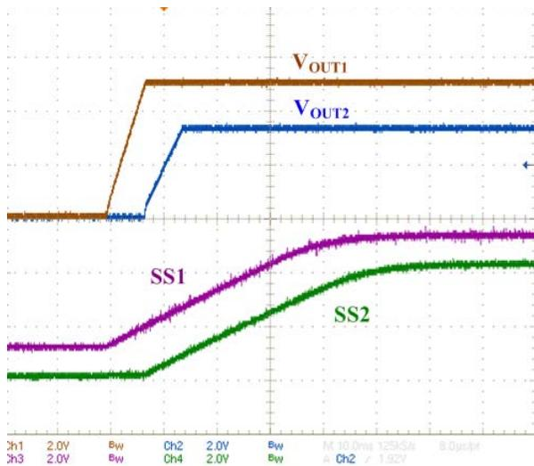
Figure 49. Sequential Mode – Power-up
