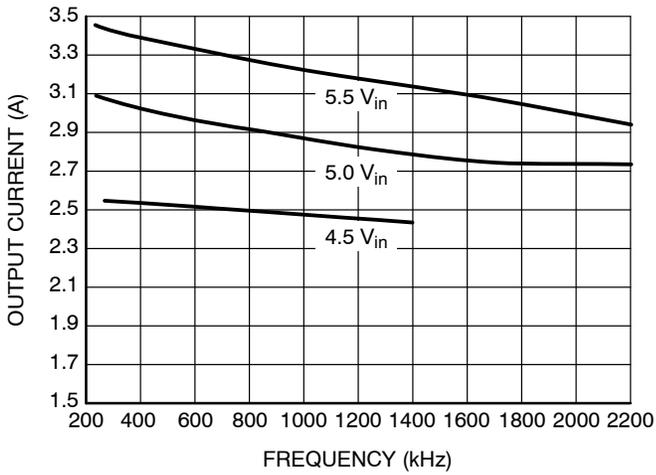
Figure 31. Maximum Currents vs. Operating Frequency due to Toff min limitations 1.8 Vout
