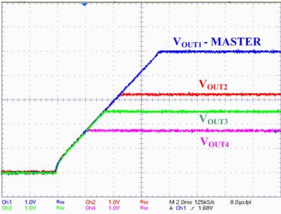
Figure 58. Tracking Mode of Four Outputs – Power-up
