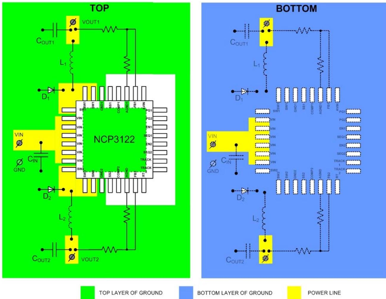
Figure 75. Typical Layout Diagram
