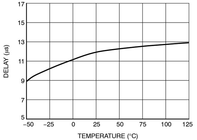
Figure 18. Power Good Falling Delay vs. Temperature
