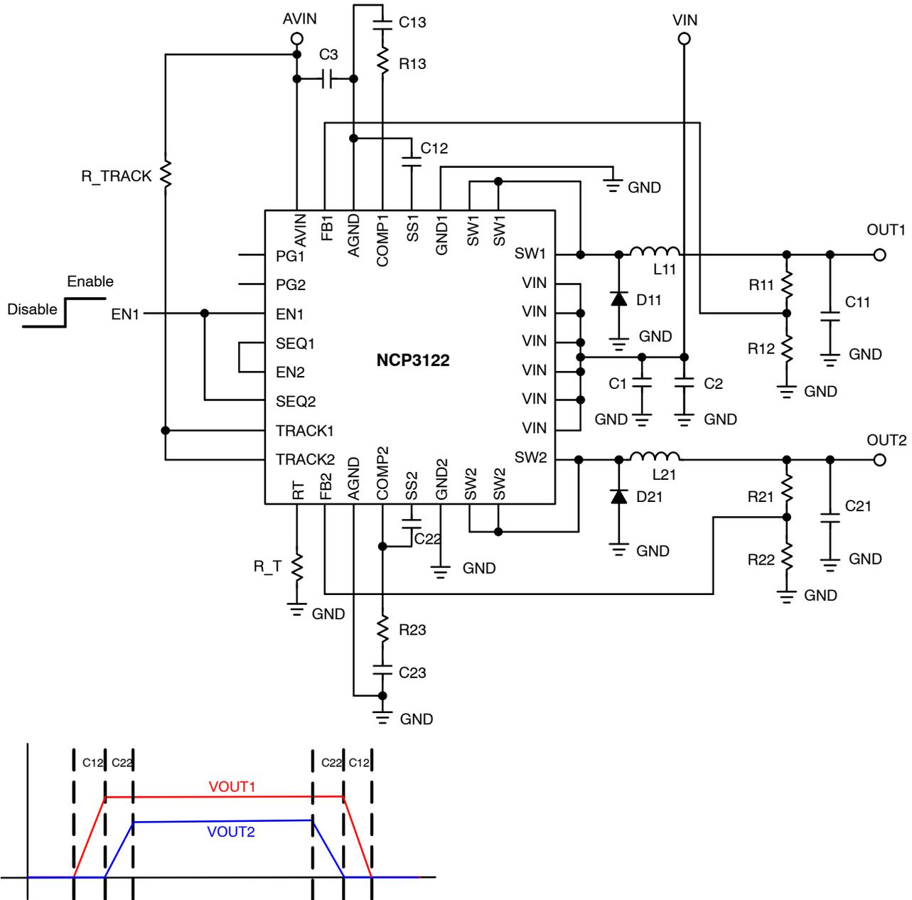
Figure 46. Sequential Configuration
