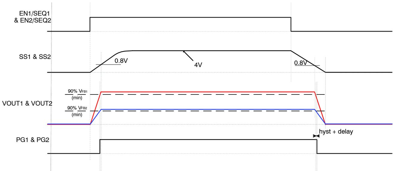
Figure 41. Typical Behavior of Ratiometric Sequencing Mode
