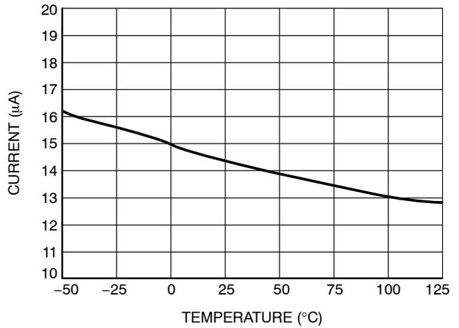
Figure 22. SEQ Internal Pull-down Current vs. Temperature
