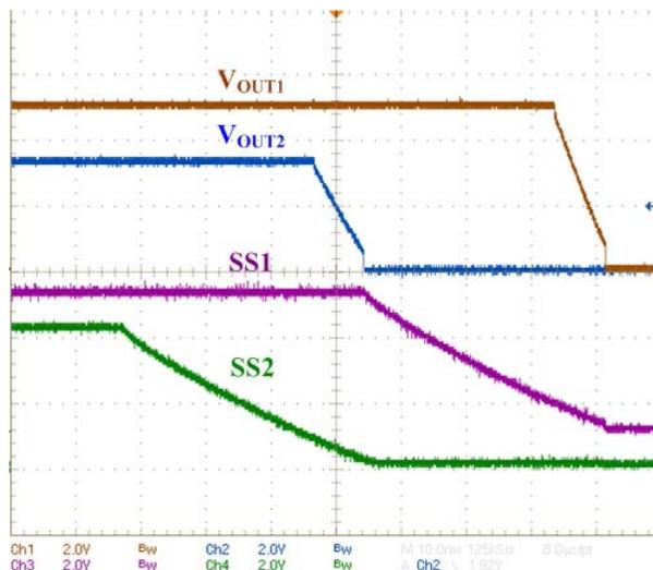
Figure 50. Sequential Mode – Power-down
