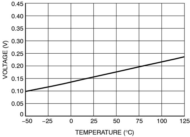
Figure 19. Power Good Saturation Voltage vs. Temperature
