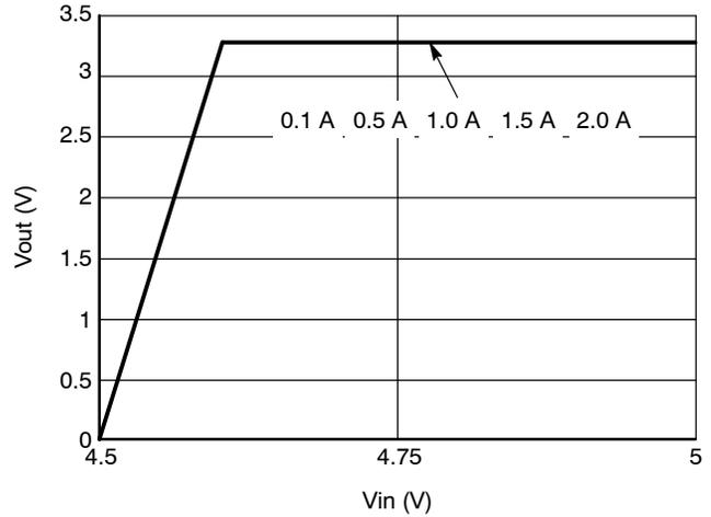
Figure 34. Minimum Input Voltage 3.3 Vout, 350 kHz
