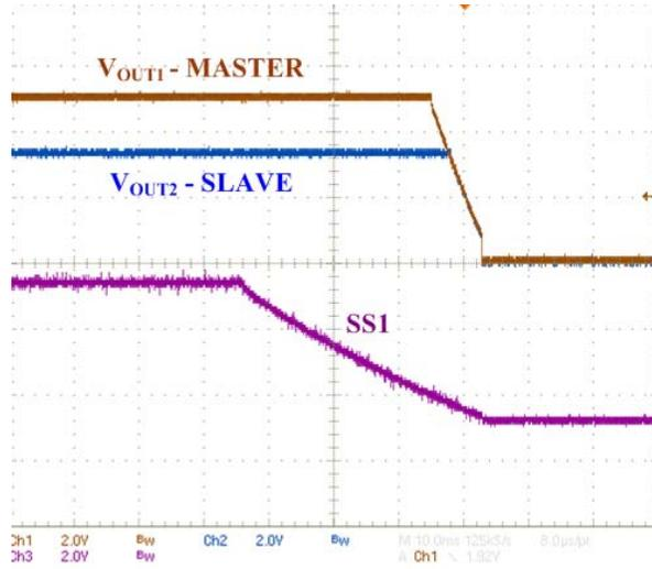
Figure 57. Tracking Mode – Power-down
