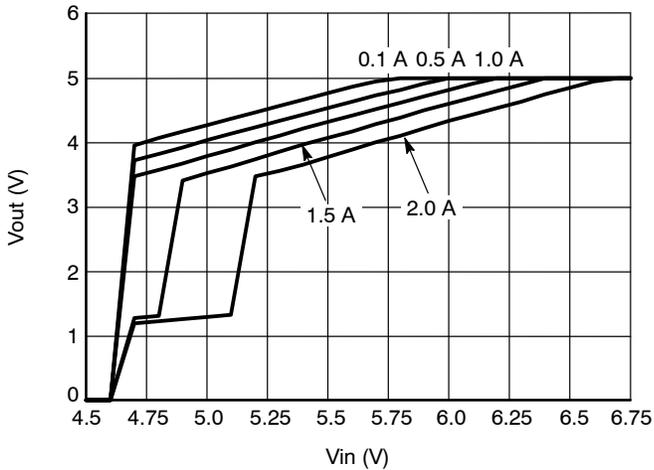
Figure 35. Minimum Input Voltage 5 Vout, 2.1 MHz
