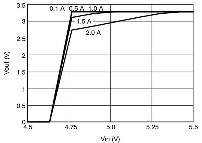
Figure 36. Minimum Input Voltage 3.3 Vout, 2.1 MHz
