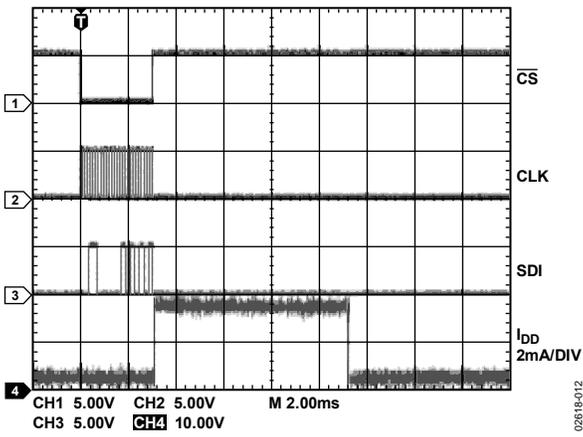
Figure 12.  $I_{DD}$  vs. Time (Save) Program Mode
