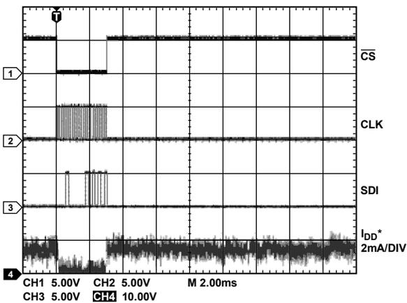
\*SUPPLY CURRENT RETURNS TO MINIMUM POWER CONSUMPTION IF COMMAND INSTRUCTION 0 (NOP) IS EXECUTED IMMEDIATELY AFTER COMMAND INSTRUCTION 1 (READ EEMEM).
