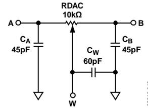
Figure 43. RDAC Circuit Simulation Model for RDACx = 10 kΩ
