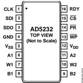
Figure 4. Pin Configuration
