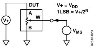
Figure 23. Potentiometer Divider Nonlinearity Error (INL, DNL)
