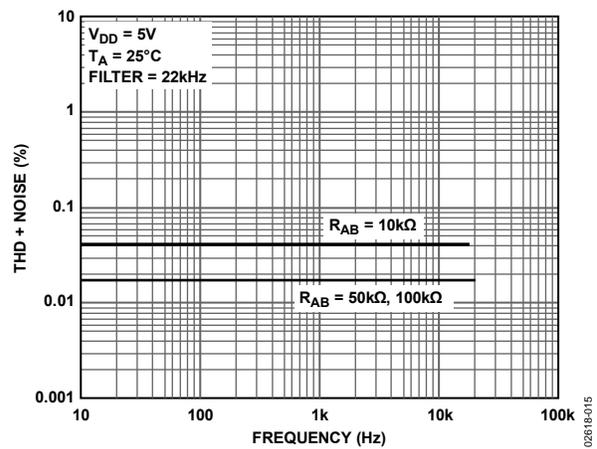
Figure 15. Total Harmonic Distortion + Noise vs. Frequency
