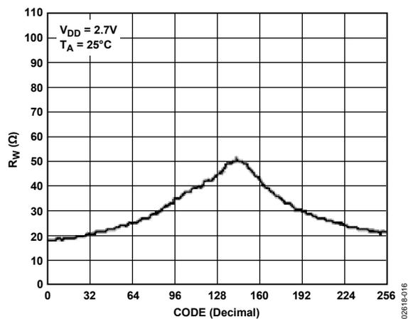
Figure 16. Wiper On Resistance vs. Code
