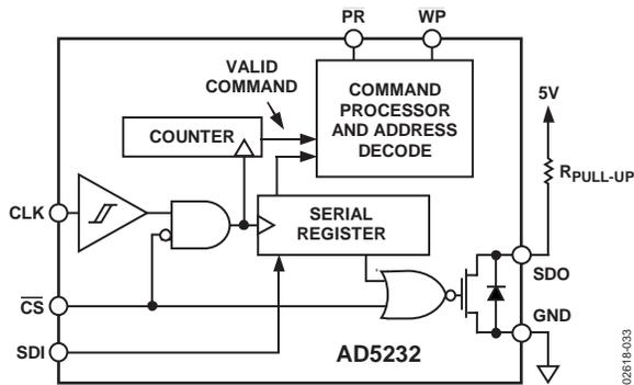
Figure 33. Equivalent Digital Input/Output Logic
