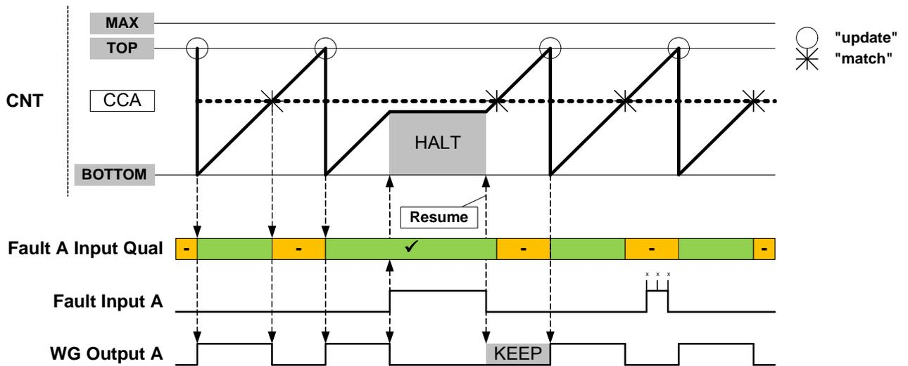
If the restart action is enabled, the timer/counter is halted as long as the fault condition is present and restarted when the fault condition is no longer present, as shown in Figure 16-12 on page 216. The compare channel output A is clamped to inactive level as long as the timer/counter is halted. Note that in RAMP2 mode of operation, when a new timer/counter cycle starts, the cycle index will change automatically.
