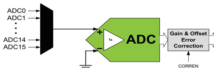
In unsigned mode, the negative input is connected to half of the voltage reference ( $V_{REF}$ ) voltage minus a fixed offset. The nominal value for the offset is:
