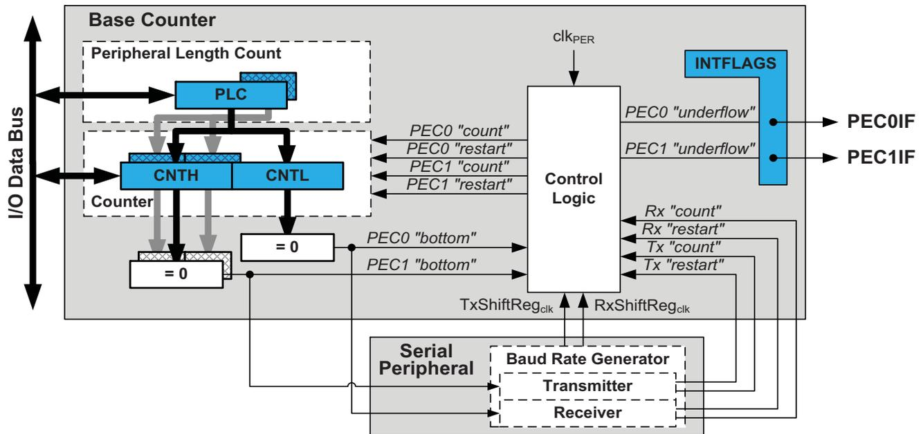
In peripheral counter configuration (PEC), the peripheral length control register (PLC) represents the TOP value and the compare is always done with the BOTTOM.
