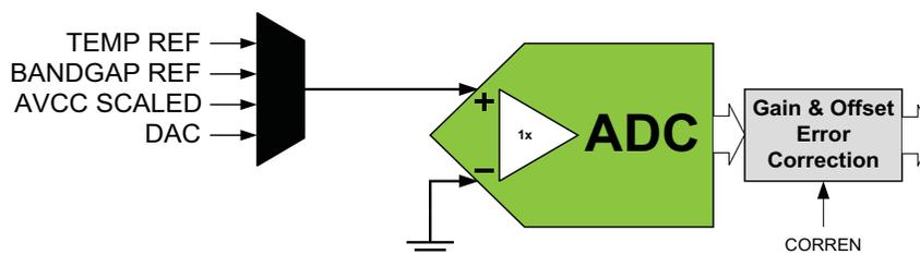
To measure the internal signals in unsigned mode, the negative input is connected to a fixed value given by the formula below, which is half of the voltage reference ( $V_{REF}$ ) minus a fixed offset, as it is for single-ended unsigned input. Refer to [Table 25-2 on page 355](#) for details.
