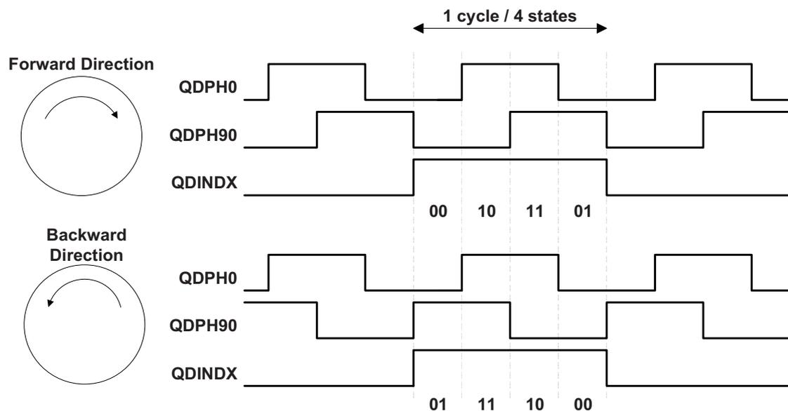
Figure 6-5 on page 86 shows typical quadrature signals from a rotary encoder. The signals QDPH0 and QDPH90 are the two quadrature signals. When QDPH90 leads QDPH0, the rotation is defined as positive or forward. When QDPH0 leads QDPH90, the rotation is defined as negative or reverse. The concatenation of the two phase signals is called the quadrature state or the phase state.
