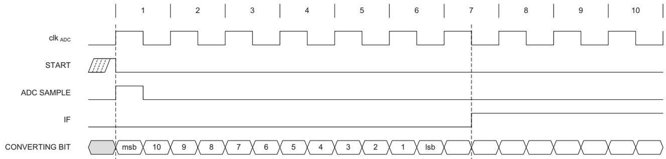
Figure 25-12. ADC Timing for One Conversion with Increased Sampling Time (SAMPVAL = 6)
