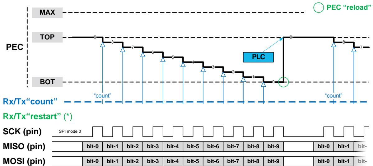
(\*) No Rx/Tx“restart”: During PEC initialization for SPI communication, set-up PEC=PLC.
