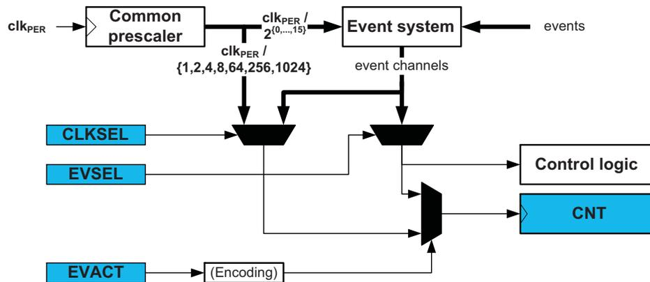
The peripheral clock is fed into a common prescaler (common for all timer/counters in a device). Prescaler outputs from 1 to 1/1024 are directly available for selection by the timer/counter. In addition, the whole range of prescaling from 1 to  $2^{15}$  times are available through the event system.
