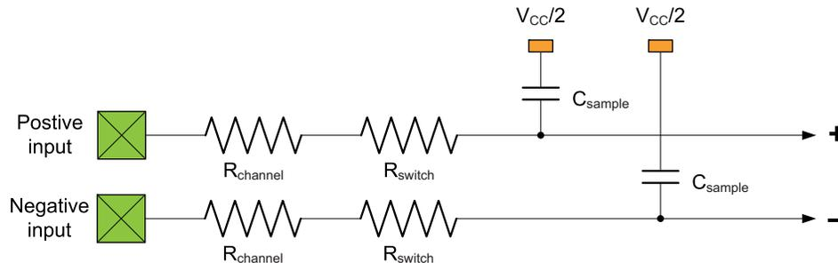
In order to achieve  $n$  bits of accuracy, the source output resistance,  $R_{source}$ , must be less than the ADC input resistance on a pin:
