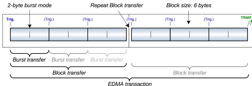
A complete EDMA read and write operation between memories and/or peripherals is called an EDMA transaction. A transaction is done in data blocks, and the size of the transaction (number of bytes to transfer) is selectable from software and controlled by the block size and repeat bit settings. Each block transfer is divided into bursts.
