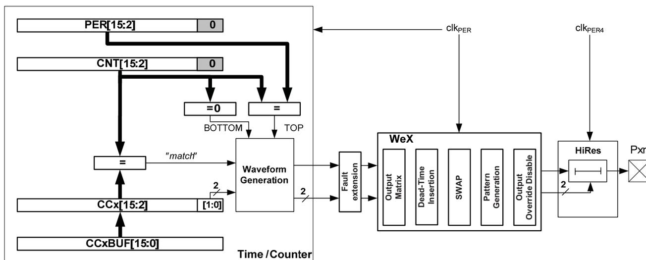
When the hi-res extension is enabled, the timer/counter must run from a non-prescaled peripheral clock. The timer/counter will ignore its two least-significant bits (lsb) in the counter, and counts by four for each peripheral clock cycle. Overflow/underflow and compare match of the 14 most-significant bits (msb) is done in the timer/counter. Count and compare of the two lsb is handled and compared in the hi-res extension running from the peripheral 4x clock.
