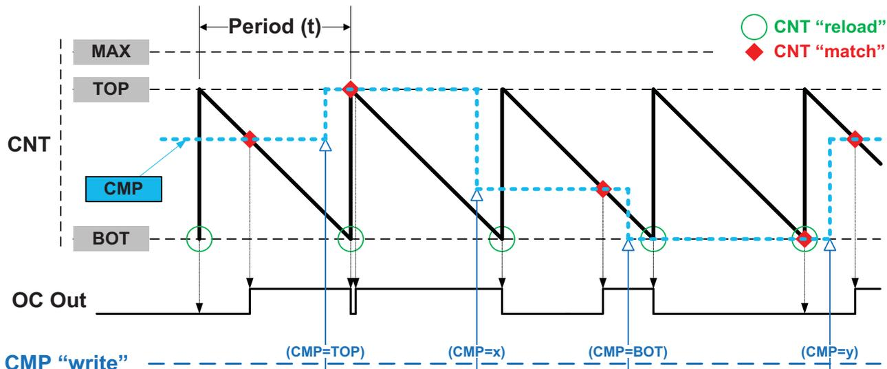
The PERCAPT register defines the PWM resolution. The minimum resolution is two bits (PERCAPT=0x03), and the maximum resolution is PERCAPT=MAX.
