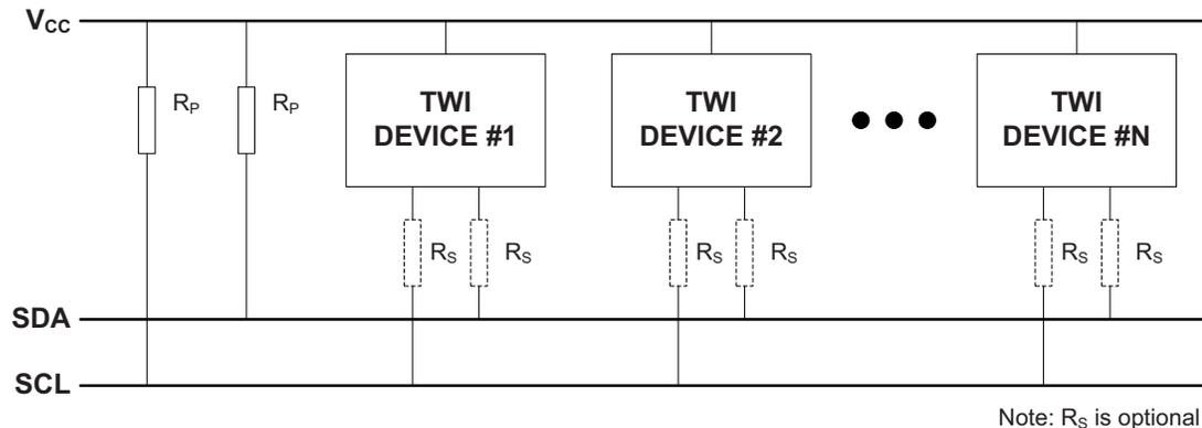
An unique address is assigned to all slave devices connected to the bus, and the master will use this to address a slave and initiate a data transaction.
