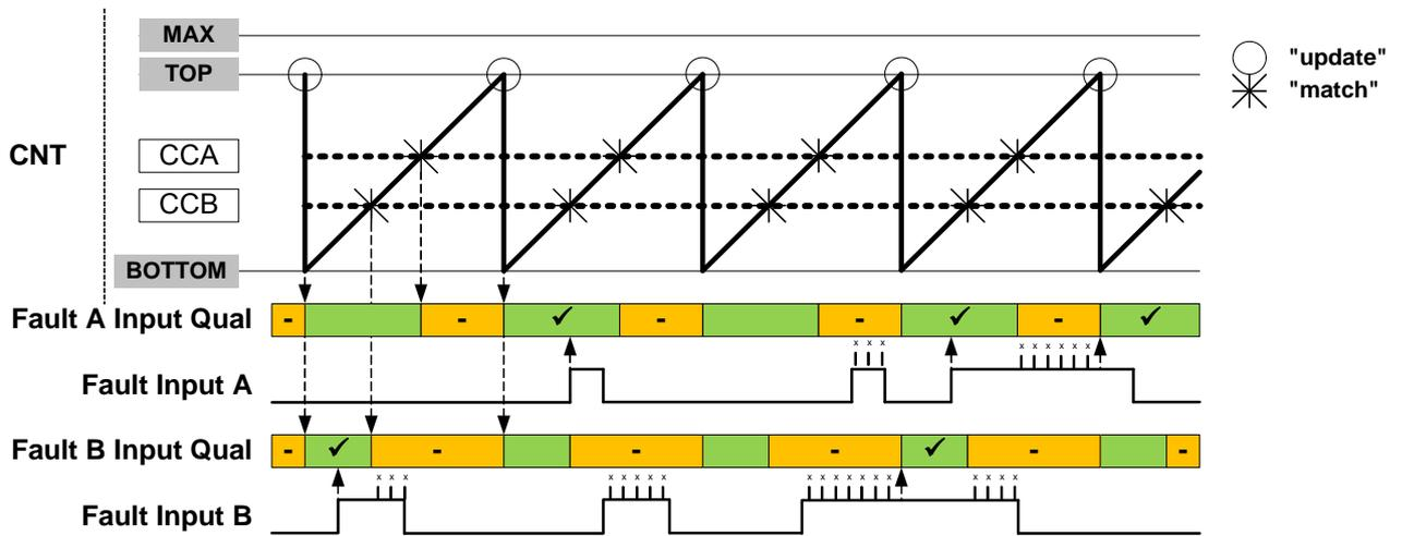
Figure 16-4. Fault Input Qualification in RAMP2 Mode with Inverted Polarity
