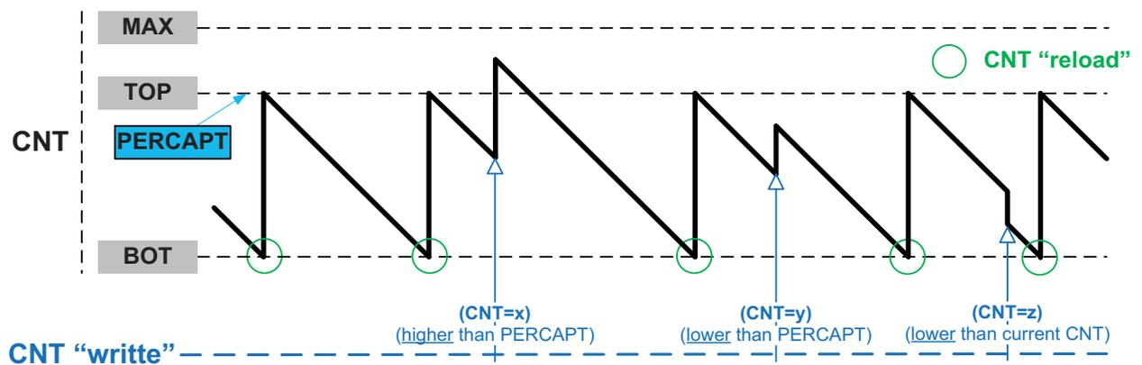
As shown in Figure 23-4, changing the counter value while the counter is running is possible. Write accesses have higher priority than count, clear, or reload and will be immediate.
