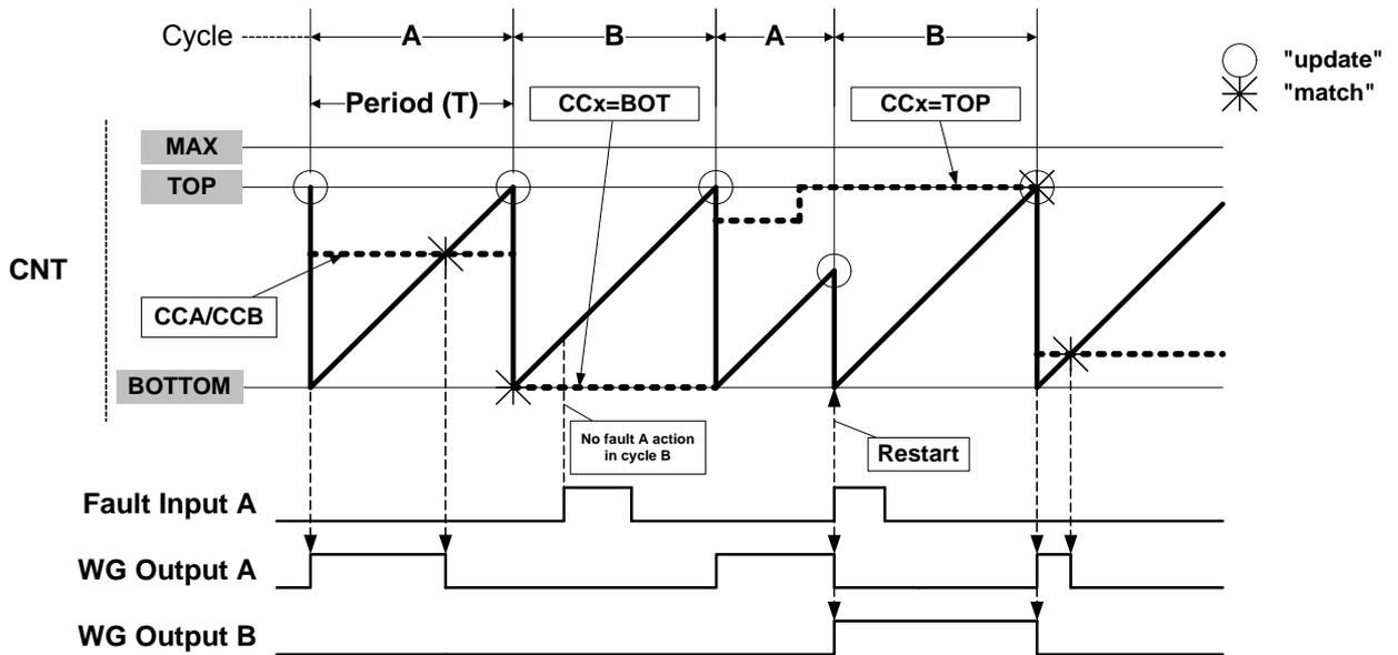
The Control logic of the restart command is shown in Figure 16-8 below.
