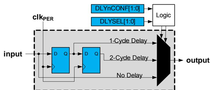
The insertion of a delay unit is selectable for each LUT, on the first of the two inputs or on the output. The insertion is decided by the application purpose, but some examples are provided:
