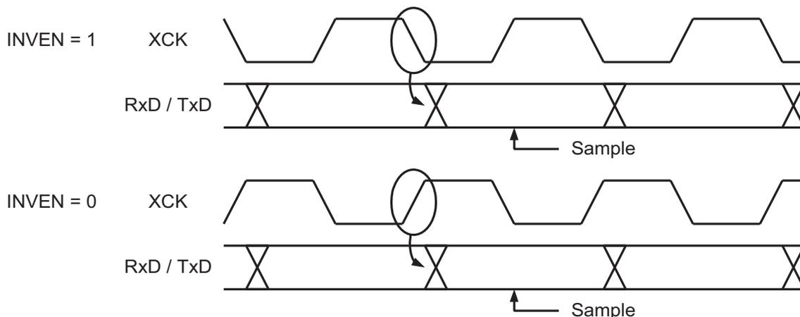
Using the inverted I/O (INVEN) setting for the corresponding XCK port pin, the XCK clock edges used for data sampling and data change can be selected. If inverted I/O is disabled (INVEN=0), data will be changed at the rising XCK clock edge and sampled at the falling XCK clock edge. If inverted I/O is enabled (INVEN=1), data will be changed at the falling XCK clock edge and sampled at the rising XCK clock edge. For more details, see “I/O Ports” on page 139.
