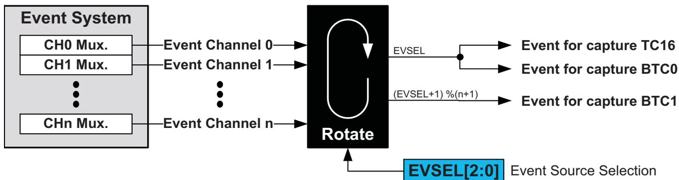
The event action setting in the timer/counter will determine the type of capture that is done. The capture operation must be enabled before capture can be done. When the capture condition occurs, the timer/counter will time-stamp the event by copying the current CNT value of the count register into the PERCAPT register.
