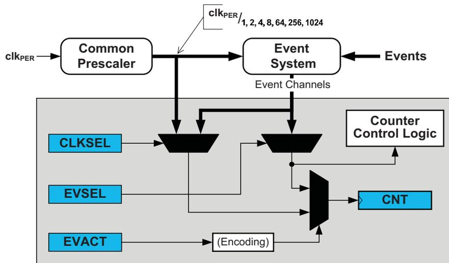
The peripheral clock is fed into the common pre-scaler (common for all timer/counters in a device). A selection of the pre-scaler outputs is directly available for both timer/counters. In addition the whole range from 1 to  $2^{15}$  times pre-scaling is available through the event system.
