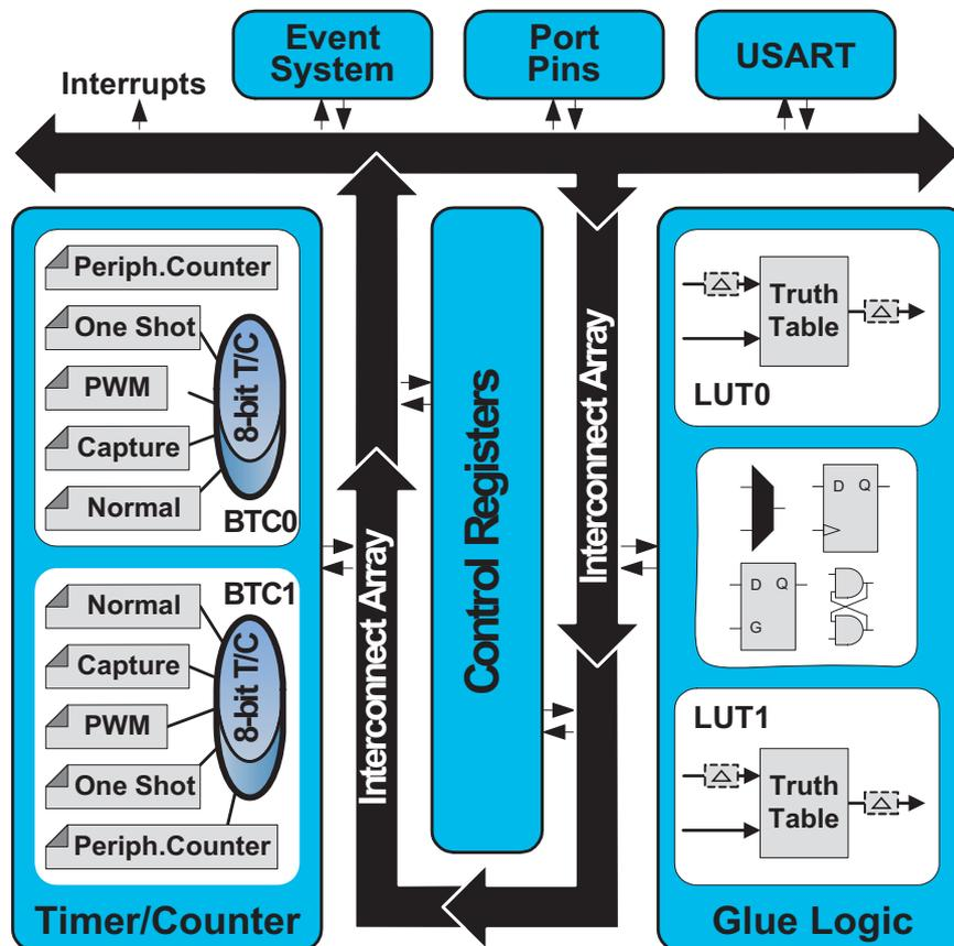
The timer/counter configuration allows for two 8-bit timer/counter usage. Each timer/counter supports normal, input capture, continuous and one shot pulse width modulations (PWM), with common flexible clock selections and event channels. By cascading the two 8-bit timer/counters, the XMEGA custom logic (XCL) offers a 16-bit timer/counter.
