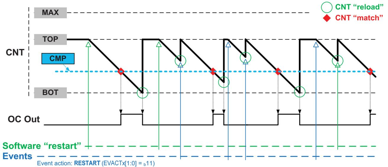
Figure 23-12. Timer/counter in 1SHOT Configuration with STOPSTART Command
