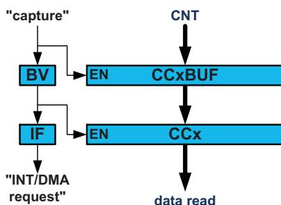
Both the CCx and CCxBUF registers are available as an I/O register. This allows initialization and bypassing of the buffer register and the double buffering function.
