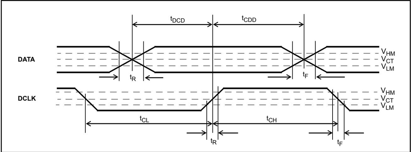
Figure 12 - DATA and DCLK Mode 0 Output Timing
