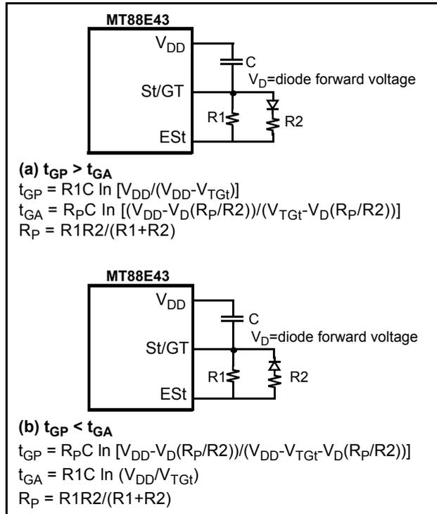
Figure 5 - Guard Time Circuits with Unequal Times
