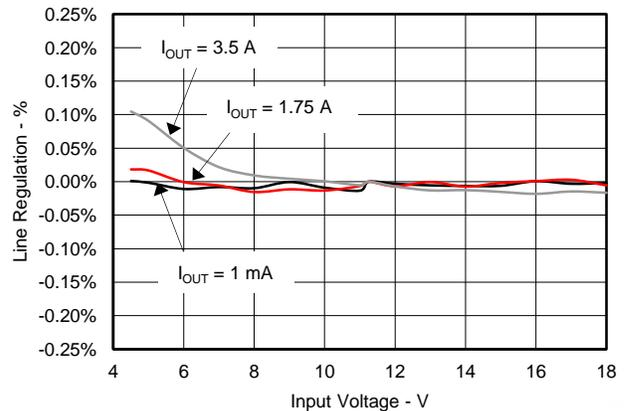
Figure 10. Line Regulation,  $V_{\text{OUT}2} = 1.0\text{ V}$ , Eco-mode = OFF
