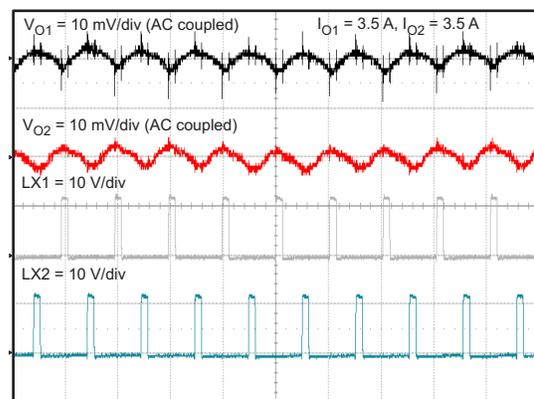
Figure 12. Output Ripple at 3.5 A, Forced PWM
