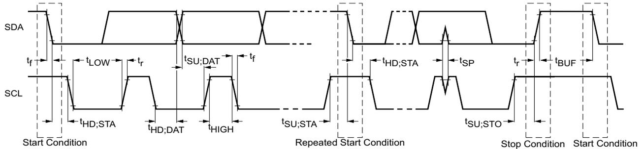
**Figure 28. I<sup>2</sup>C Interface Timing Diagram**
