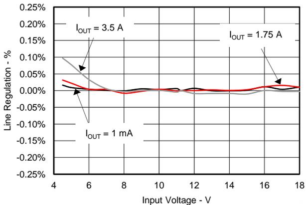
Figure 9. Line Regulation,  $V_{\text{OUT}1} = 1.0\text{ V}$ , Eco-mode = OFF
