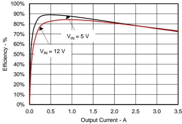
Figure 1. 1-V Efficiency
