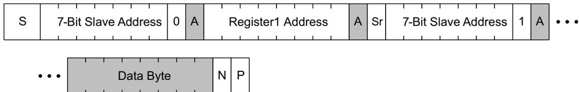
**Figure 30. I<sup>2</sup>C Read Data Format**
