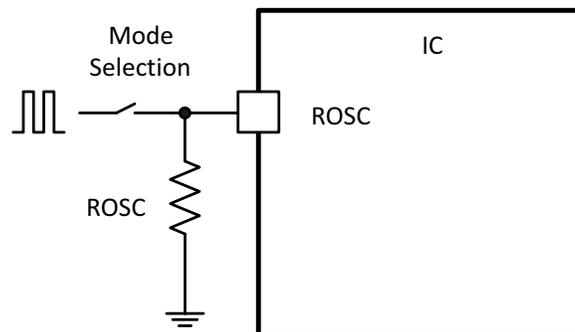
Figure 27. Resistor Mode and Synchronization Mode
