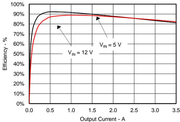
Figure 3. 1.8-V Efficiency
