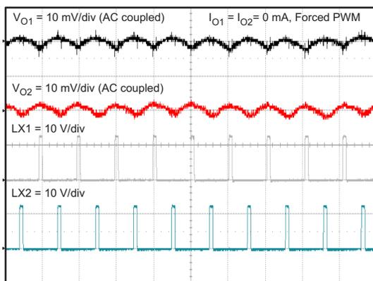
Figure 11. Output Ripple at 0 A, Forced PWM
