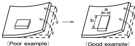
(2) Components location on PCB separation
