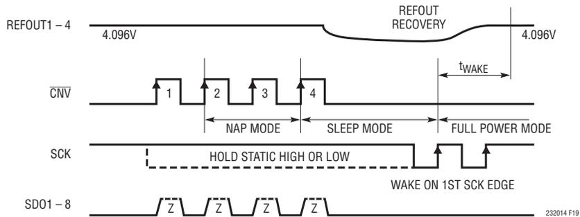
Figure 19. CMOS Mode SLEEP and WAKE Using SCK
