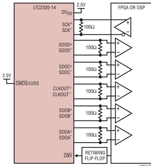
Figure 22. LTC2320-14 Using the LVDS Interface
