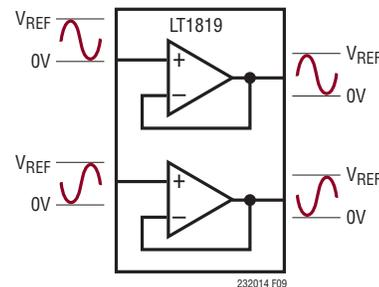
Figure 9. LT1819 Buffering a Fully-Differential Signal Source
