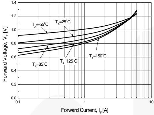
**Figure 1. Forward Voltage vs Forward Current (Per diode)**
