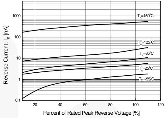
**Figure 2. Typical Reverse Current Characteristics (Per Diode)**
