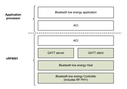
Figure 23. nRF8001 ACI connectivity
