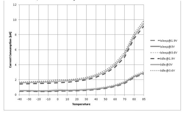
Figure 16. Current consumption in  $I_{idle}$  and  $I_{sleep}$  with DC/DC converter not active
