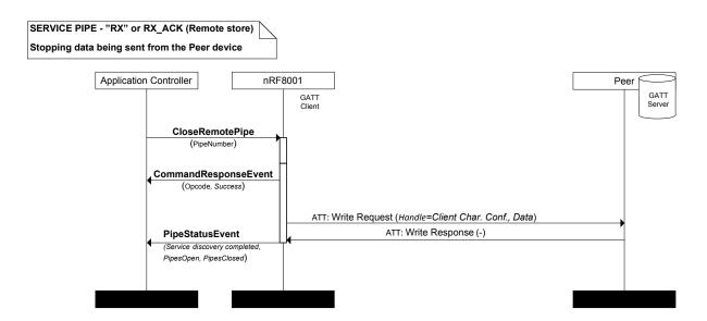
Figure 33. Receive pipe closing; data stored remotely
