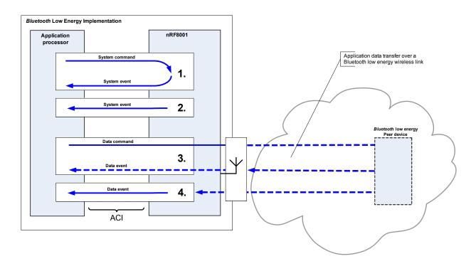
Figure 24. ACI operating principle
