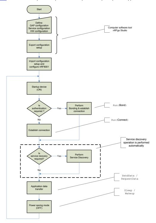
Figure 52. Normal configuration and connection establishment procedure (example)
