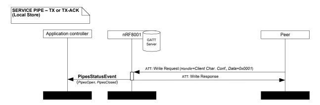
Figure 27. Transmit pipe opening; local data storage
