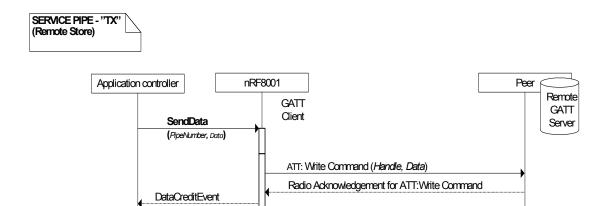
Figure 31. Data transfer on a transmit pipe; acknowledgment enabled and data stored remotely
