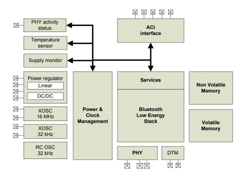
Figure 1. nRF8001 block diagram
