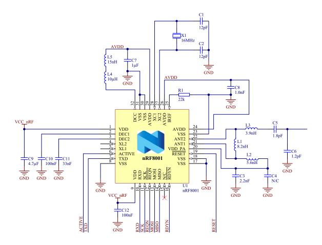
Figure 21. nRF8001 schematic, with DC/DC converter enabled
