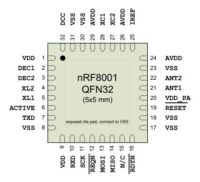
Figure 3. nRF8001 pin assignment (top view)
