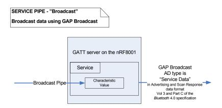
Figure 41. Broadcasting data using GAP broadcast
