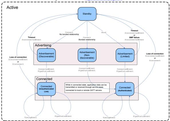
Figure 49. Active mode operation state machine
