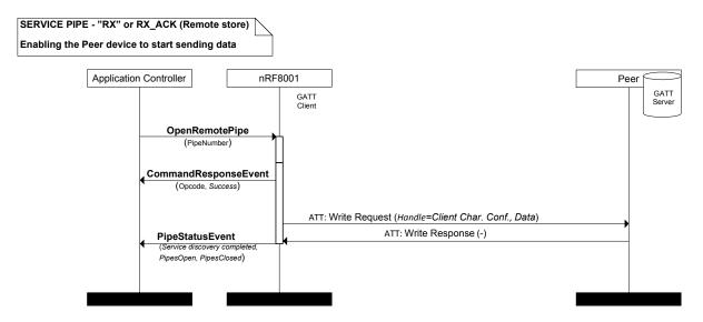
Figure 32. Receive pipe opening; data stored remotely
