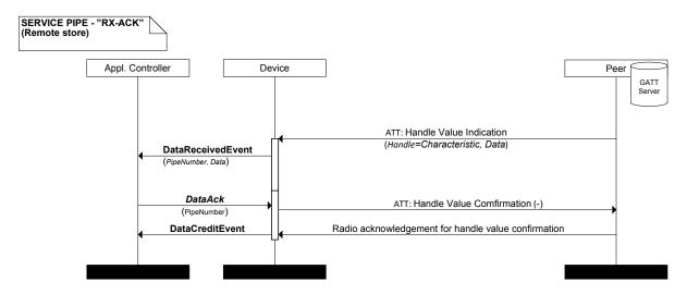
Figure 38. Data transfer on a receive pipe; acknowledgment enabled and data stored remotely
