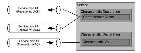
Figure 26. Service pipes assigned to characteristics under a service
