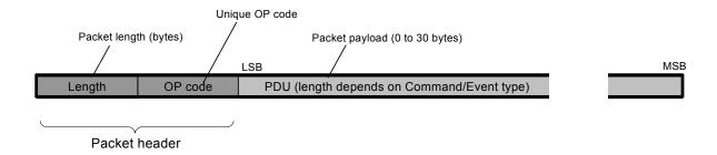
Figure 25. ACI packet structure
