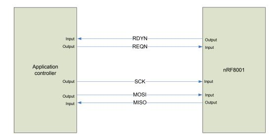
Figure 7. ACI interface between application controller and nRF8001
