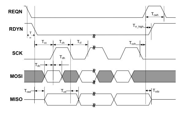
Figure 12. Application controller initiated packet SPI timing
