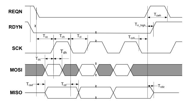
Figure 13. nRF8001 initiated packet SPI timing
