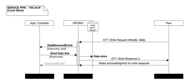
Figure 35. Data transfer on a receive pipe; acknowledgment enabled and data stored locally
