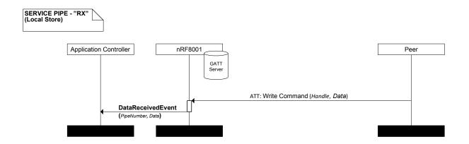
Figure 34. Data transfer on a receive pipe; data stored locally
