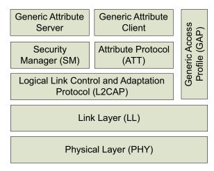
Figure 2. Bluetooth low energy layers implemented in nRF8001
