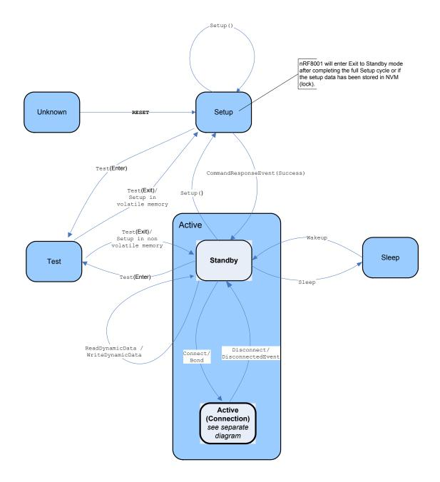
Figure 45. State Machine: Transition between operational modes<sup>3</sup>
