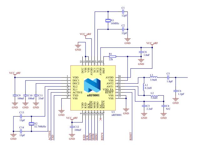
Figure 22. nRF8001 schematic, with DC/DC converter disabled
