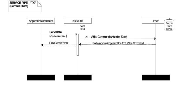
Figure 30. Data transfer on a transmit pipe; data stored remotely
