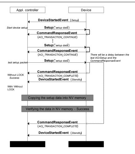
Figure 46. Setup procedure MSC
