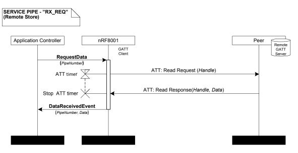
Figure 40. Data transfer on a receive pipe after data request received, data stored remotely
