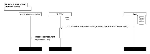
Figure 37. Data transfer on a receive pipe; data stored remotely
