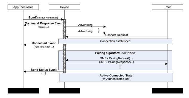
Figure 50. Bonding procedure MSC
