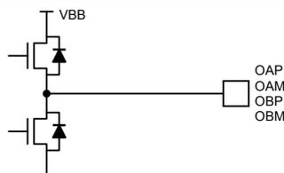
Figure 19i: Phase Outputs
