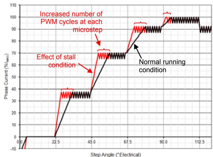
Figure 3. Effect of stall condition on current rise
