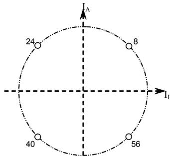
Figure 8: Full-step Phase Diagram Using STEP Input
