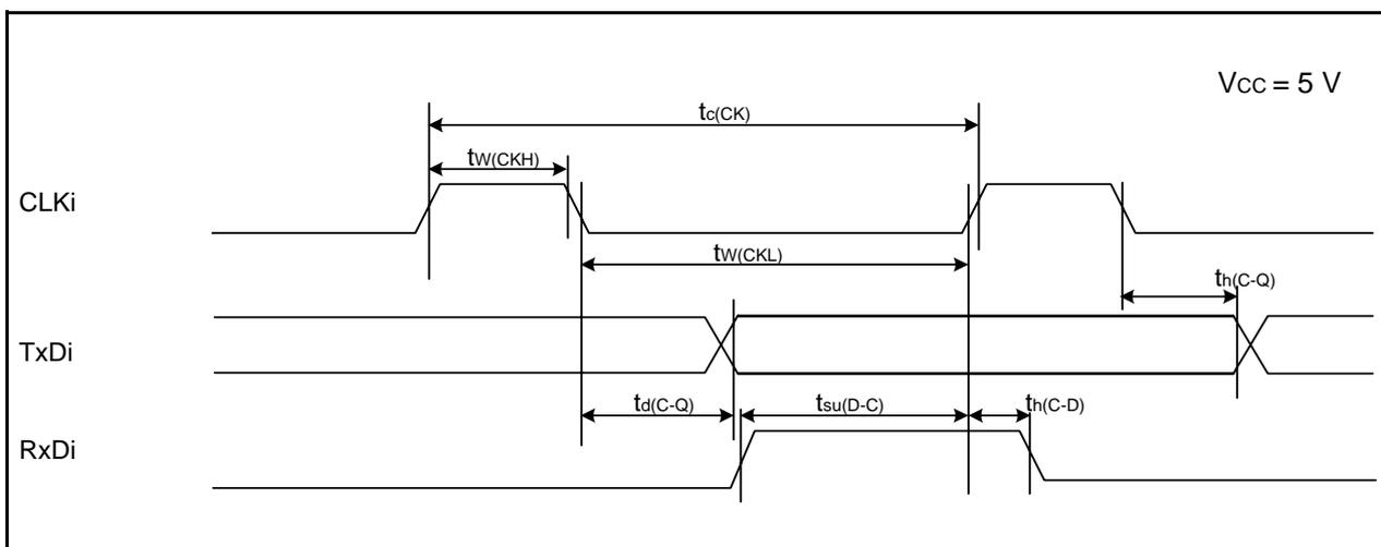
**Figure 5.7 Serial Interface Timing Diagram when Vcc = 5 V**
