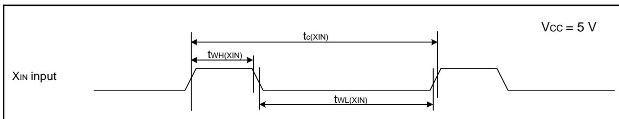
**Figure 5.4 XIN Input Timing Diagram when  $V_{CC} = 5\text{ V}$** **Table 5.15 CNTR0 Input, CNTR1 Input,  $\overline{INT1}$  Input**
