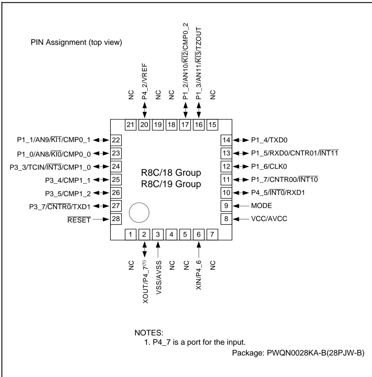
Figure 1.6 Pin Assignments for PWQN0028KA-B Package (Top View)
