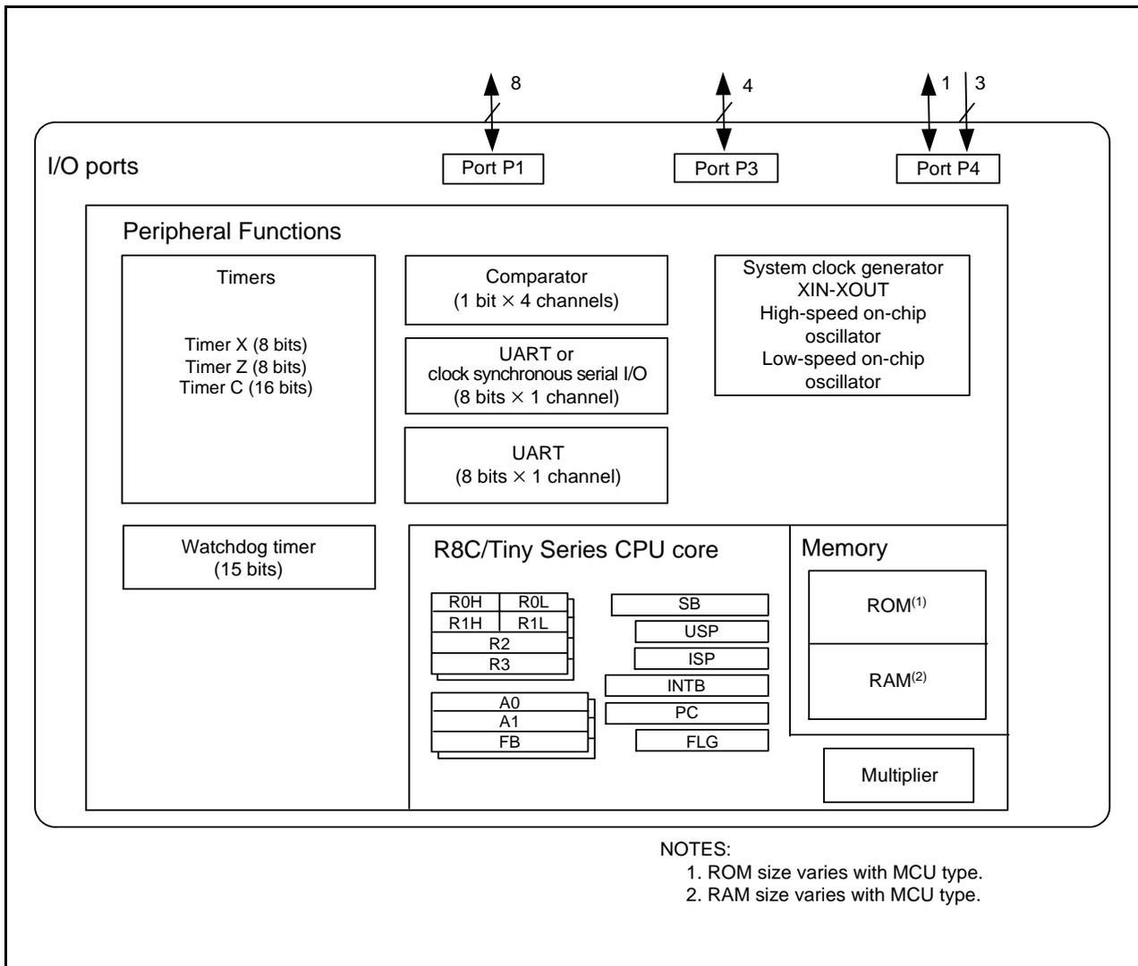
Figure 1.1 Block Diagram
