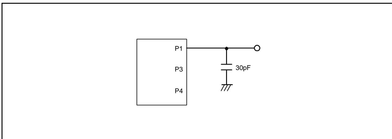
**Figure 5.1 Port P1, P3, and P4 Measurement Circuit**
