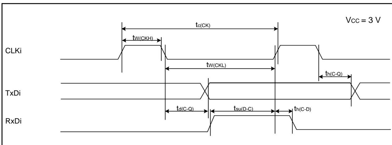
**Figure 5.12 Serial Interface Timing Diagram when Vcc = 3 V**
