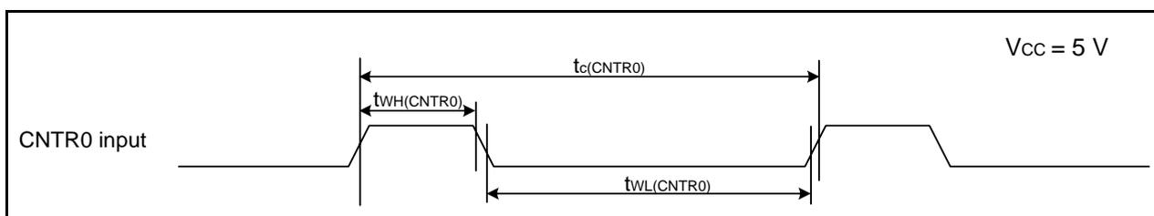
**Figure 5.5 CNTR0 Input, CNTR1 Input,  $\overline{INT1}$  Input Timing Diagram when  $V_{CC} = 5\text{ V}$** **Table 5.16 TCIN Input,  $\overline{INT3}$  Input**
