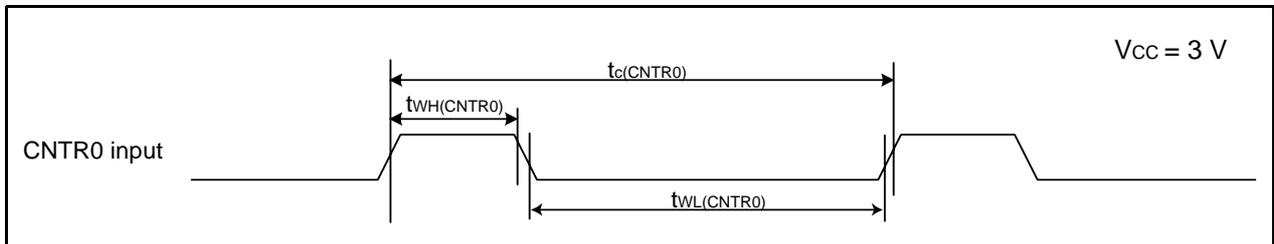
**Figure 5.10 CNTR0 Input, CNTR1 Input,  $\overline{INT1}$  Input Timing Diagram when  $V_{CC} = 3\text{ V}$** **Table 5.23 TCIN Input,  $\overline{INT3}$  Input**
