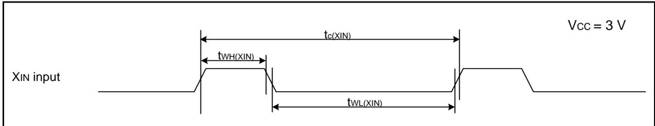
**Figure 5.9 XIN Input Timing Diagram when  $V_{CC} = 3\text{ V}$** **Table 5.22 CNTR0 Input, CNTR1 Input,  $\overline{INT1}$  Input**
