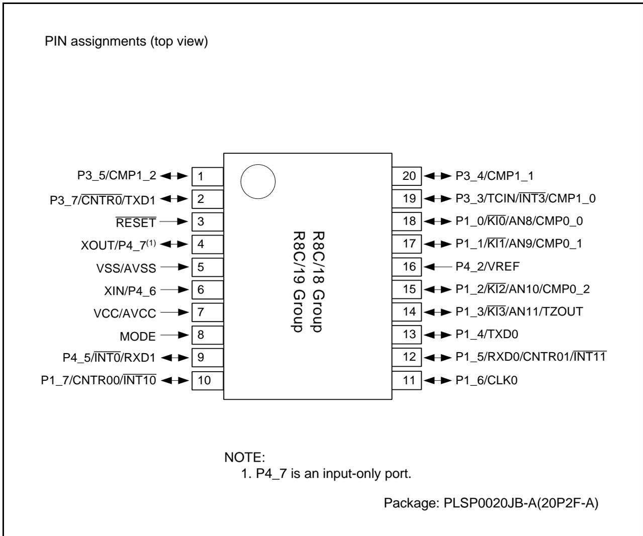
Figure 1.4 Pin Assignments for PLSP0020JB-A Package (Top View)
