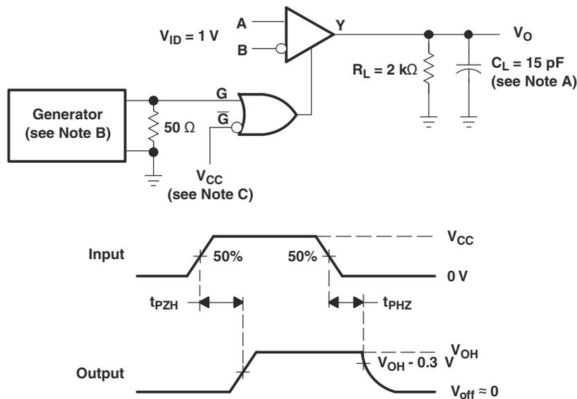
A.  $C_L$  includes probe and jig capacitance.
