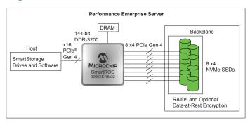
Ultra-high RAID 5 performance and capacity, 8 x4 optional data-at-rest encryption.
