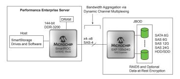
SmartROC provides remote connectivity or expansion to lower speed targets such as SAS-3 and SATA through its DCMenabled SAS-4 links to the SAS-4 SXP 24G expander.
