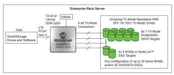
The tri-mode capability and x1 bifurcation along with new industry standards enable the universal bay architecture without sacrificing server density or performance.
