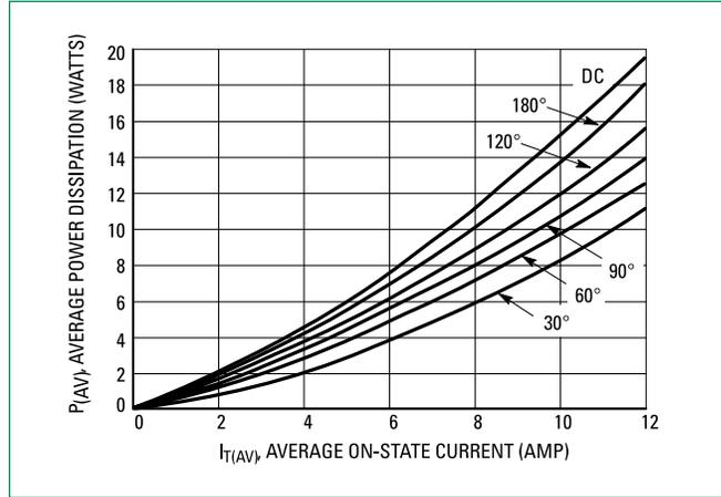
**Figure 3. On-State Characteristics**
