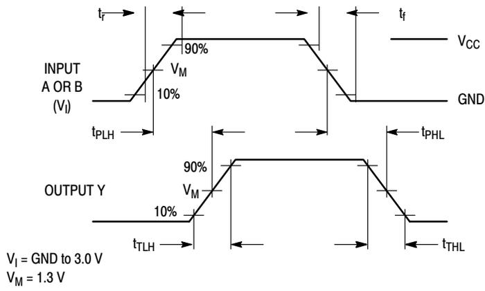
**Figure 1. Switching Waveforms**
