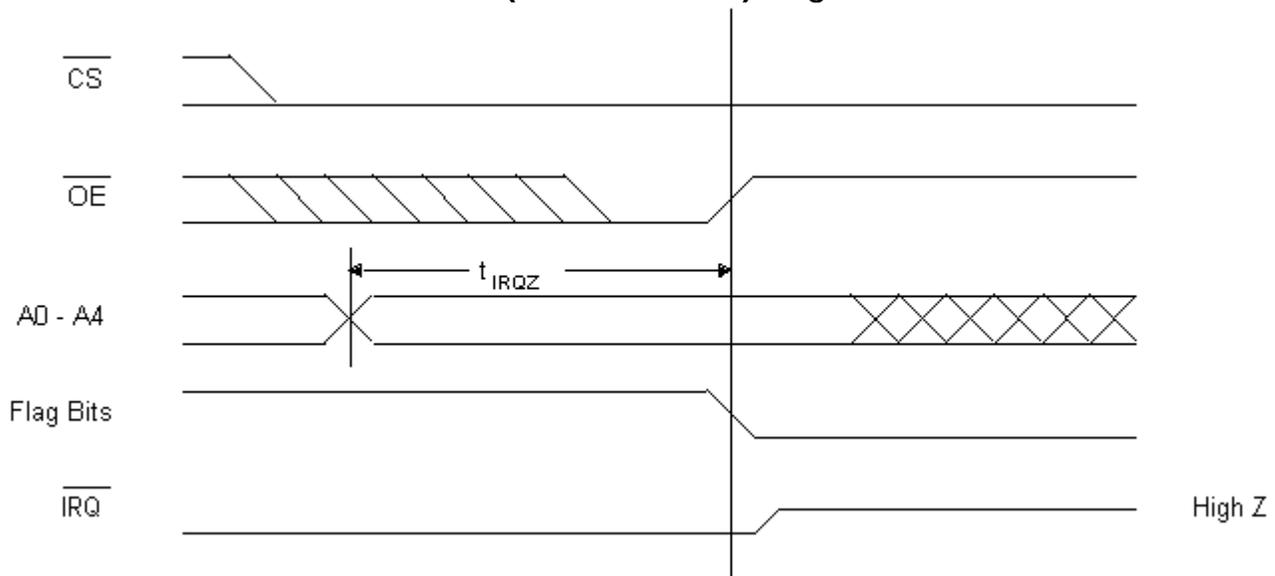
**IRQ AND FLAG WAVEFORMS ( $\overline{\text{CS}}$  RELATED) Figure 2c**
