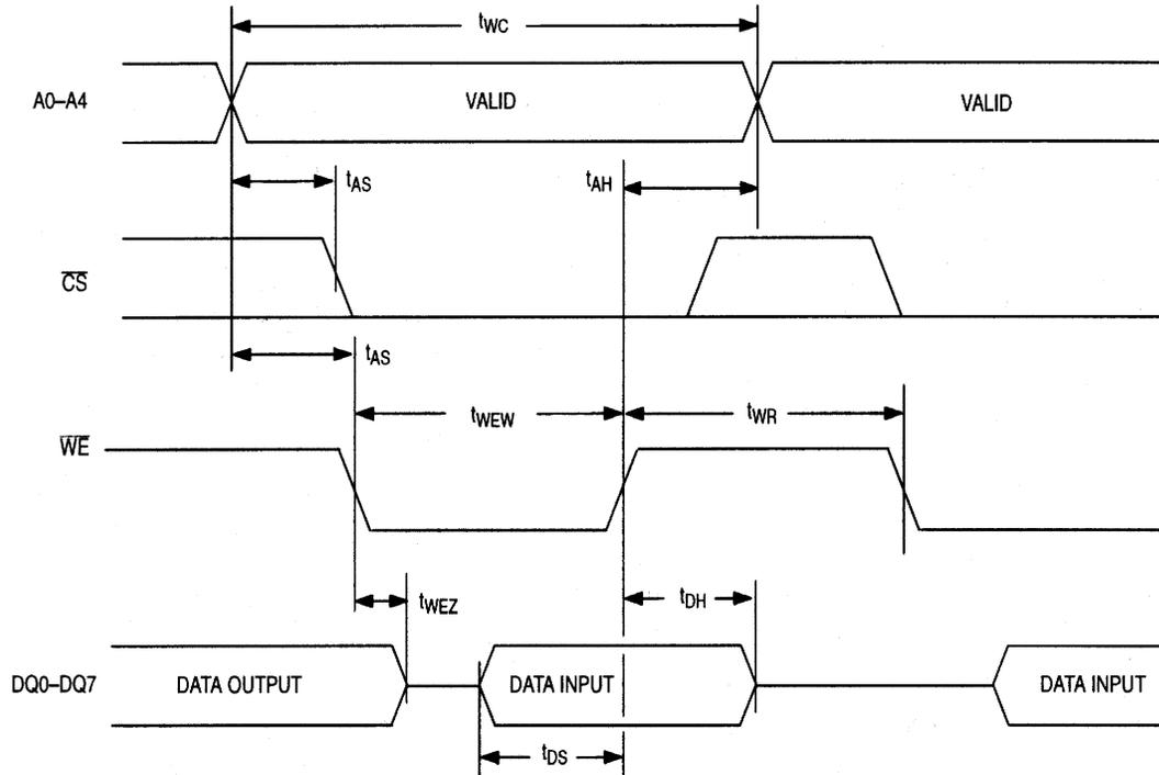
**WRITE CYCLE TIMING, CHIP ENABLE CONTROLLED Figure 5**
