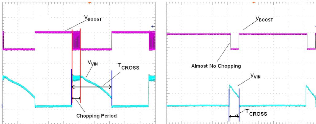
**Figure 10. Chopper Operation (Trailing Edge Dimmer Mode)**
