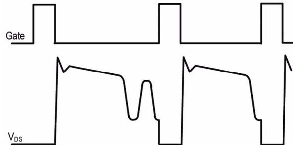
Turning on at the lowest  $V_{DS}$  generates lowest  $dV/dt$ ; thus valley mode switching can also reduce EMI. To limit the switching frequency range, the CY8CLEDAC02 can skip valleys (as shown in the first cycle in Figure 13) when the switching frequency becomes too high.
