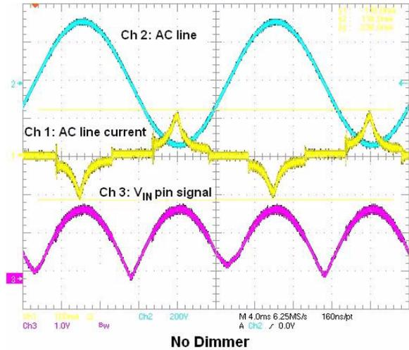
Figure 20. Inrush and AC Peak Current (Leading Edge)
