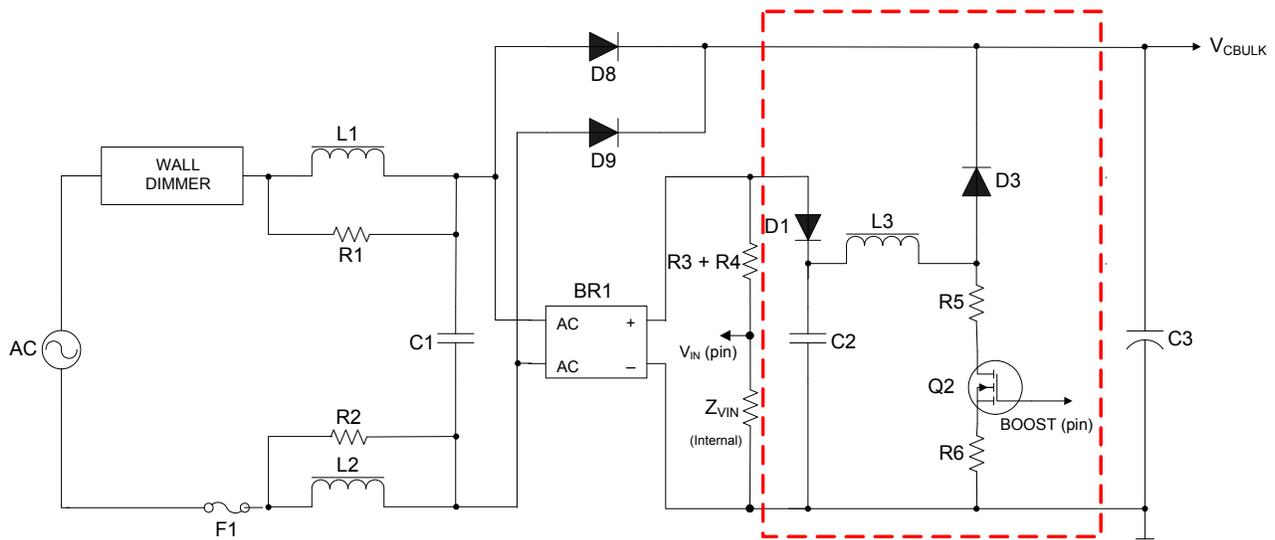
**Figure 9. Chopper Operation (Leading Edge Dimmer Mode)**
