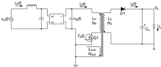
To tightly regulate output current, information about the load current needs to be accurately sensed. To achieve CC regulation, this information can be derived indirectly by sensing the primary current.
