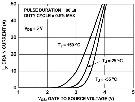
**Figure 5. Transfer Characteristics**
