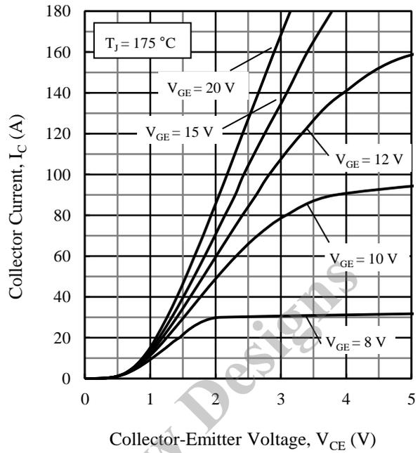
Figure 7. Output Characteristics ( $T_J = 175\text{ }^\circ\text{C}$ )
