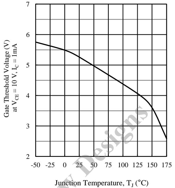
Figure 11. Gate Threshold Voltage vs. Junction Temperature
