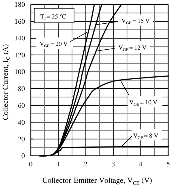
Figure 6. Output Characteristics ( $T_J = 25\text{ }^\circ\text{C}$ )
