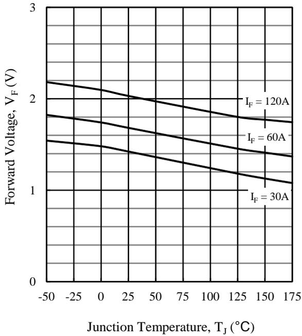
Figure 22. Diode Forward Voltage vs. Junction Temperature
