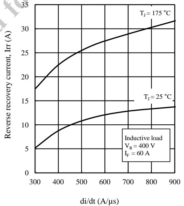
Figure 25. Diode Reverse Recovery Current vs. di/dt
