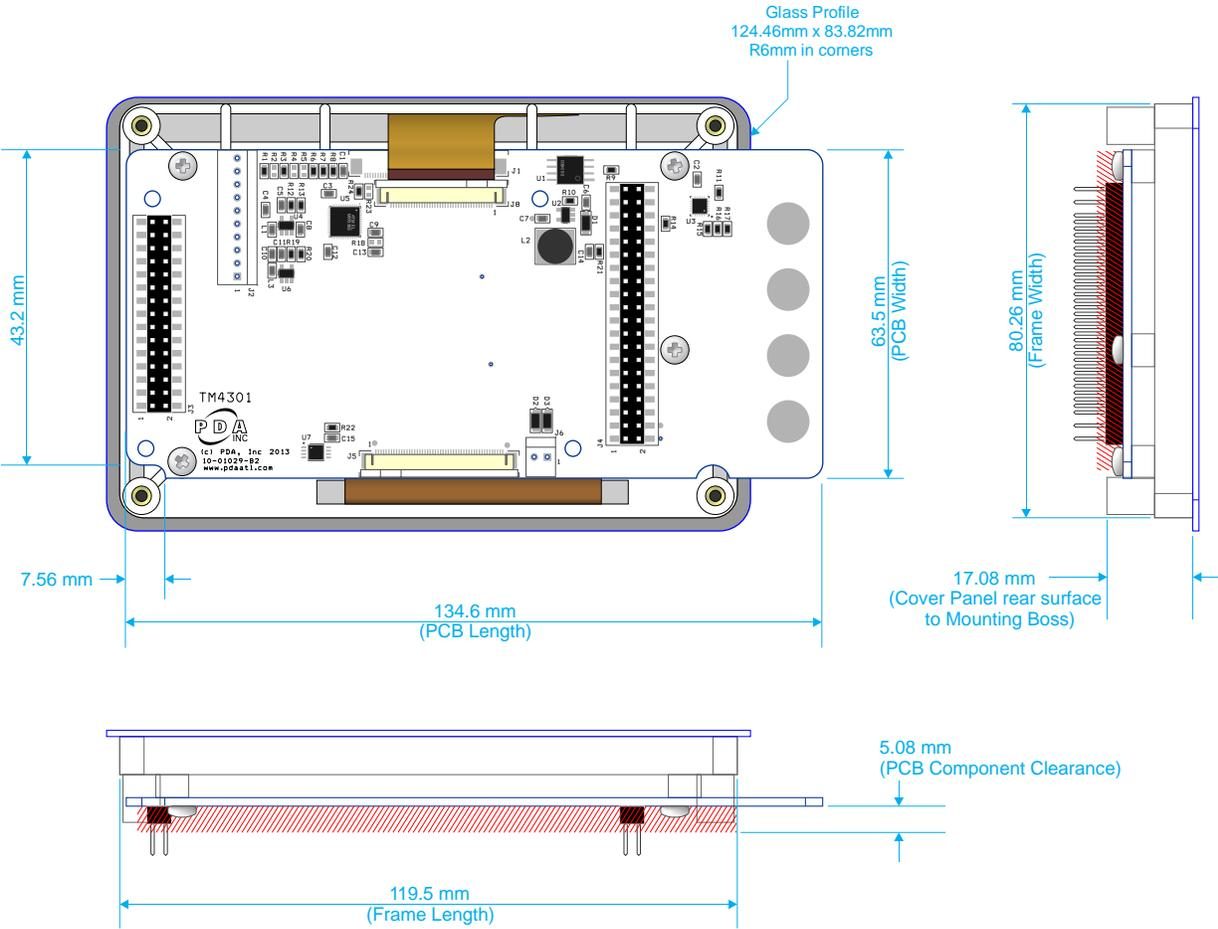
Figure 5 – Module Dimensions
