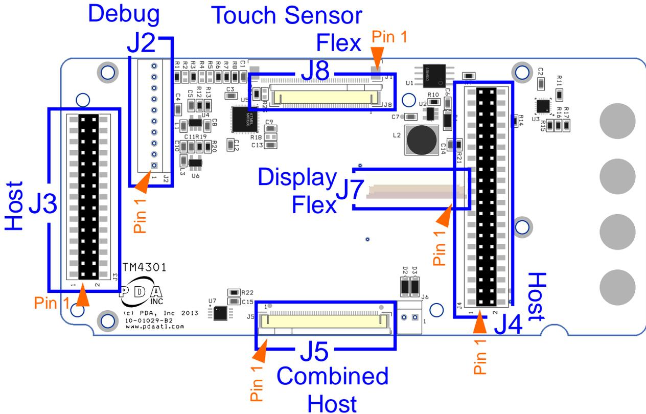
**Figure 1 - PCB Connectors**
