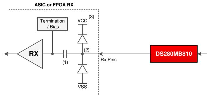
**Figure 9-2. Considerations for DC coupling to ASIC RX**
