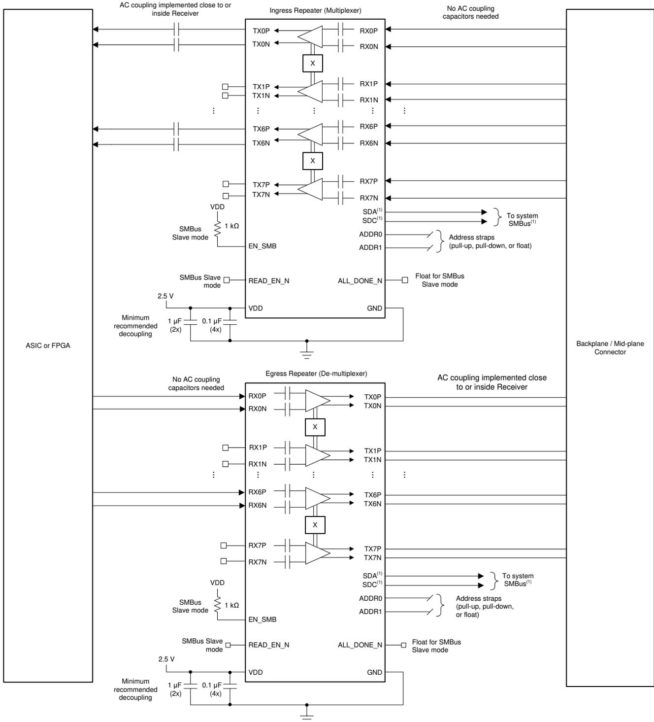
**Figure 9-4. Typical backplane and mid-plane simplified schematic**
