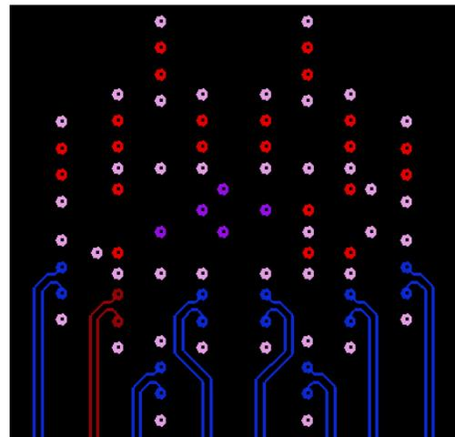
**Figure 11-2. Stripline example, Internal Signal Layer 1**
