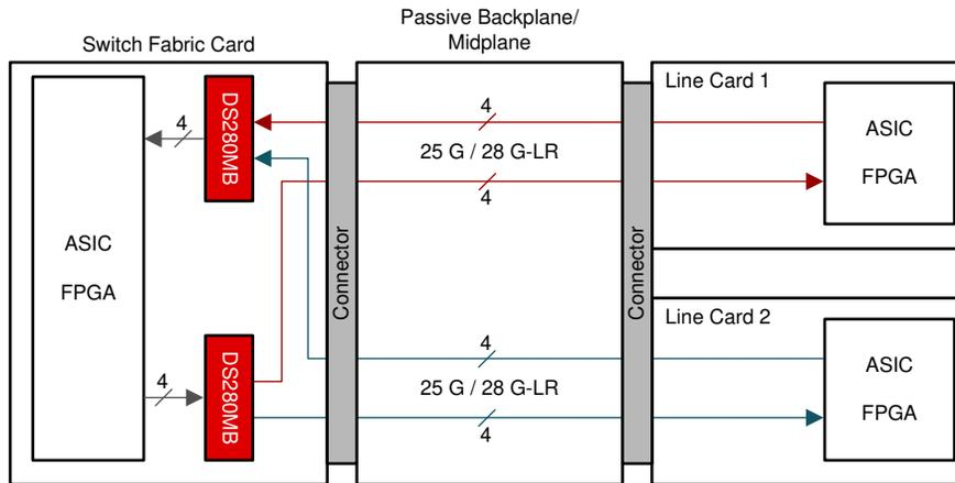
**Figure 9-3. Typical backplane and mid-plane application block diagram**
