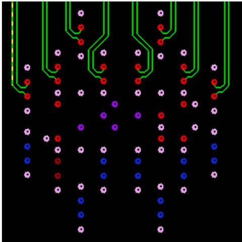
**Figure 11-3. Stripline example, Internal Signal Layer 2**
