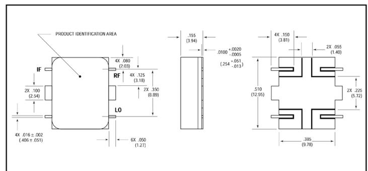
\* Dimensions are inches (millimeters) ±0.015 (0.38) unless otherwise specified.
