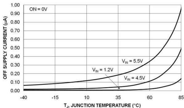
Figure 7. Off Supply Current vs. Temperature
