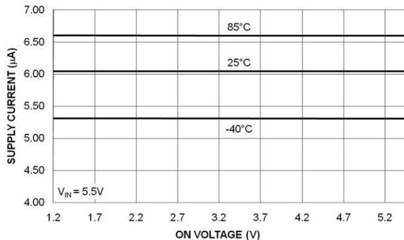
**Figure 12. Quiescent Current vs. On Voltage ( $V_{IN} = 5.5V$ )**
