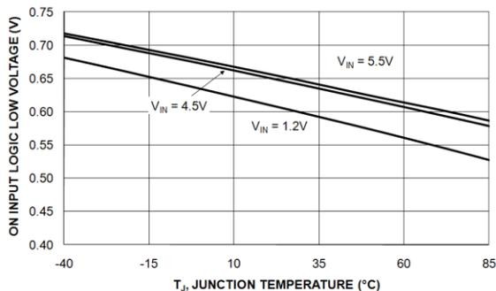
**Figure 17. On Pin Threshold Low vs. Temperature**
