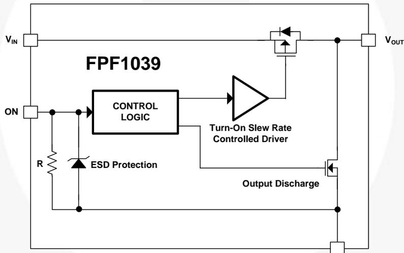
Figure 2. Functional Block Diagram
