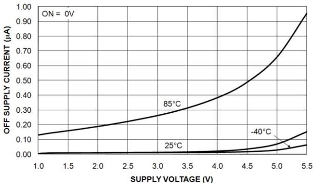
Figure 8. Off Supply Current vs. Supply Voltage
