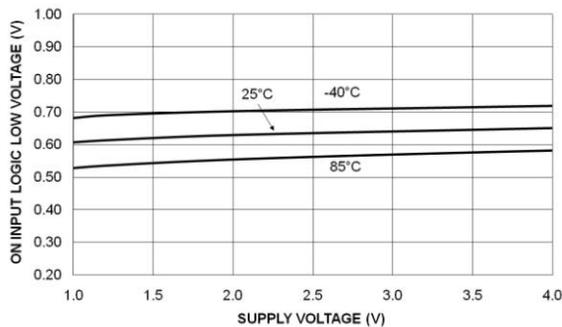
**Figure 18. On Pin Threshold Low vs.  $V_{IN}$**
