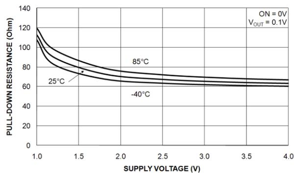
**Figure 14. Output Discharge Resistor RPD vs. Supply Voltage**
