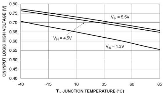
**Figure 19. On Pin Threshold High vs. Temperature**
