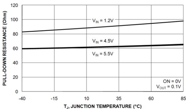
**Figure 13. Output Discharge Resistor RPD vs. Temperature**
