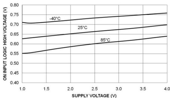
**Figure 20. On Pin Threshold High vs.  $V_{IN}$**
