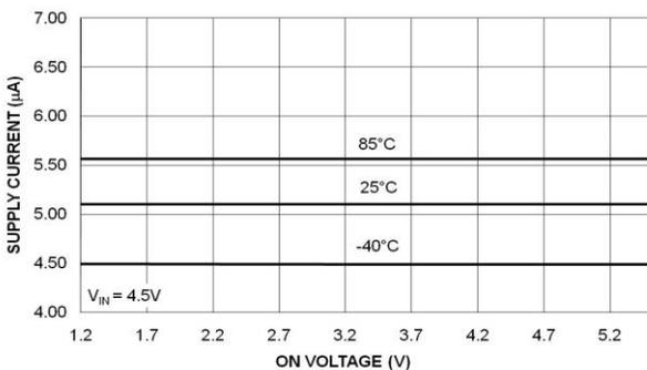
**Figure 11. Quiescent Current vs. On Voltage ( $V_{IN} = 4.5V$ )**
