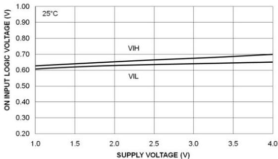
**Figure 21. On Pin Threshold vs. Supply Voltage**
