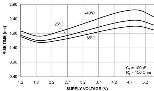
**Figure 26.**  $t_R$  vs. Supply Voltage
