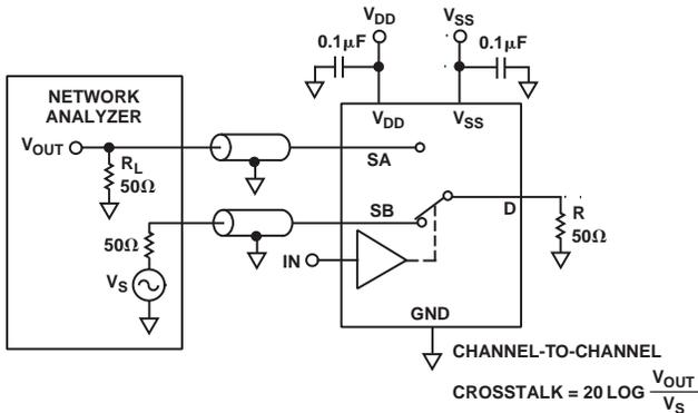
$$\text{CHANNEL-TO-CHANNEL CROSSTALK} = 20 \text{ LOG } \frac{V_{\text{OUT}}}{V_{\text{S}}}$$
