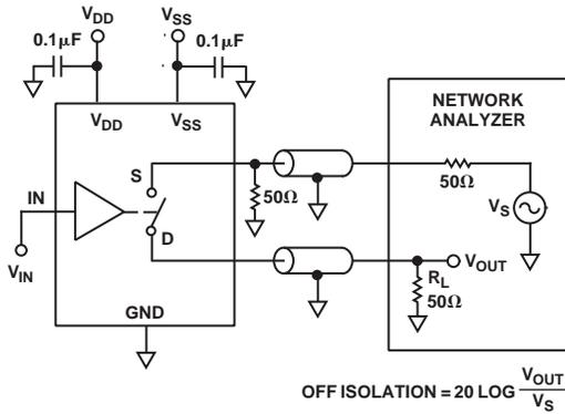
$$\text{OFF ISOLATION} = 20 \text{ LOG } \frac{V_{\text{OUT}}}{V_{\text{S}}}$$
