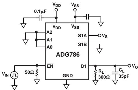
Test Circuit 5. Enable Delay,  $t_{ON}(\overline{EN})$ ,  $t_{OFF}(\overline{EN})$
