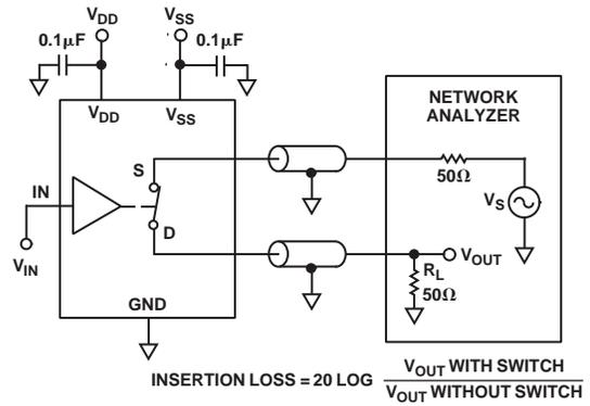
$$\text{INSERTION LOSS} = 20 \text{ LOG } \frac{V_{\text{OUT WITH SWITCH}}}{V_{\text{OUT WITHOUT SWITCH}}}$$
