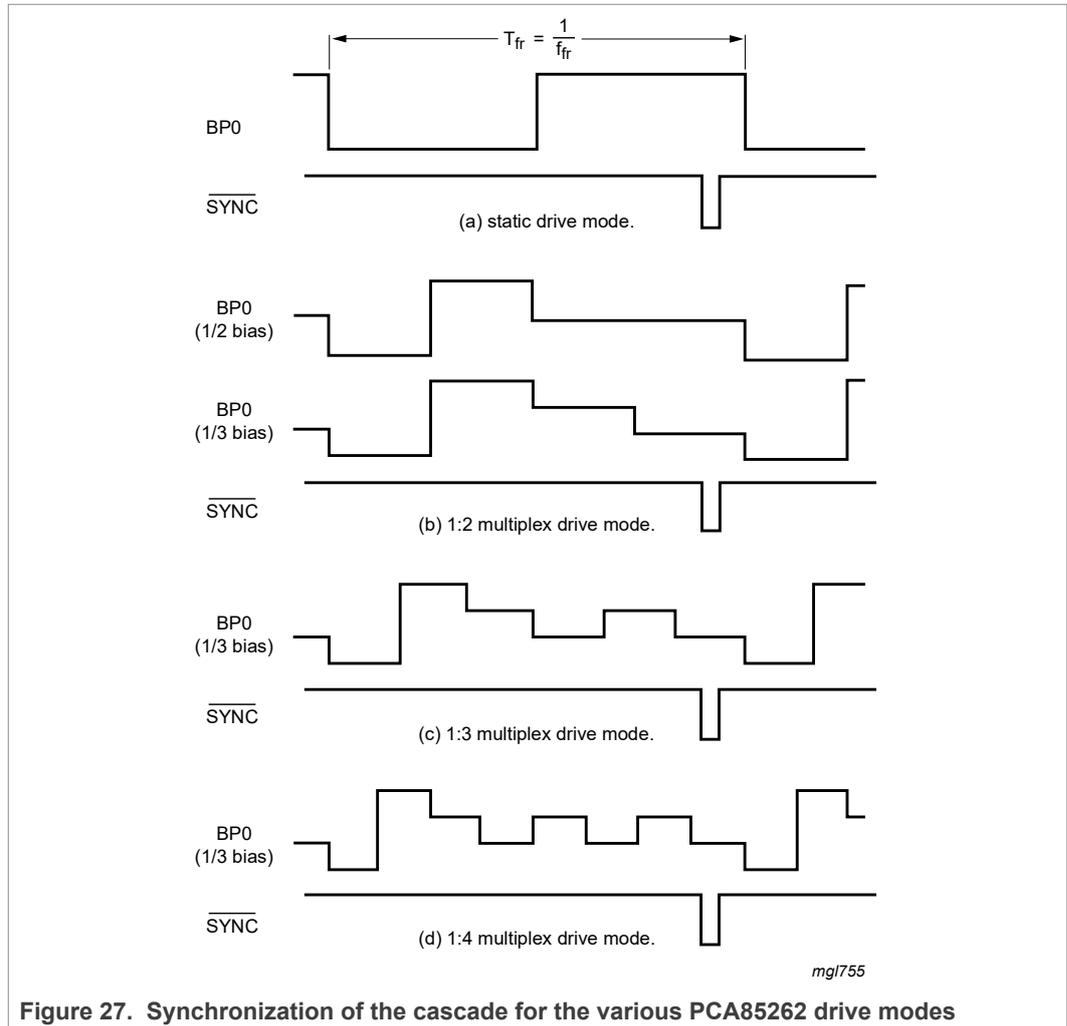
Figure 27. Synchronization of the cascade for the various PCA85262 drive modes
