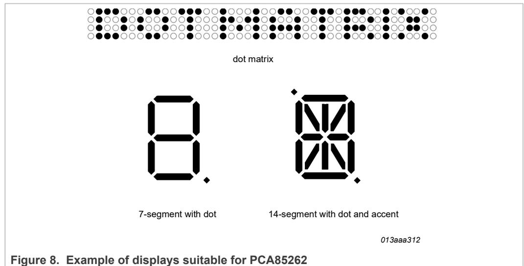
Figure 8. Example of displays suitable for PCA85262
