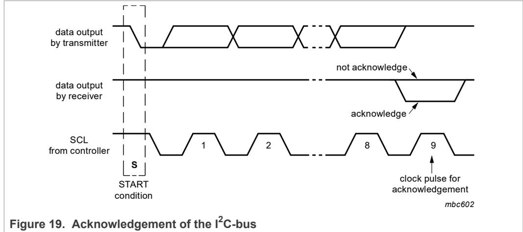
Figure 19. Acknowledgement of the I<sup>2</sup>C-bus
