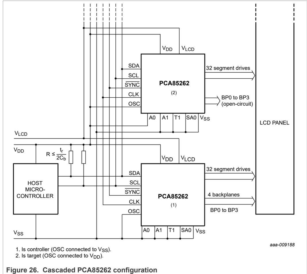
Figure 26. Cascaded PCA85262 configuration
