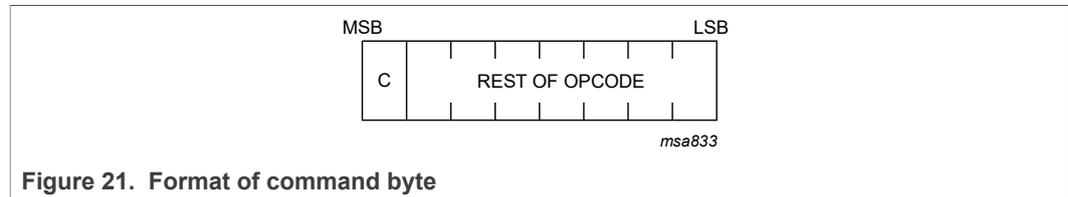
Figure 21. Format of command byte
