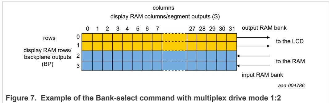
Figure 7. Example of the Bank-select command with multiplex drive mode 1:2
