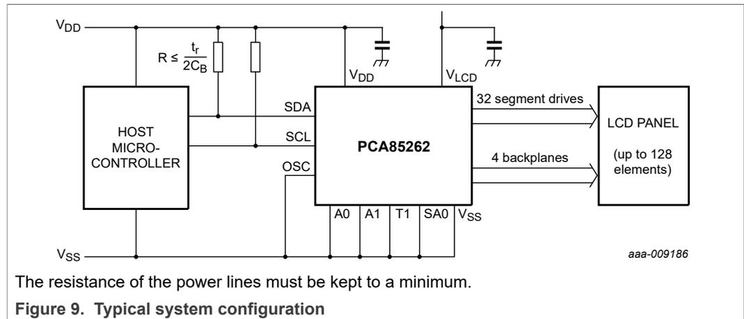
The resistance of the power lines must be kept to a minimum.
