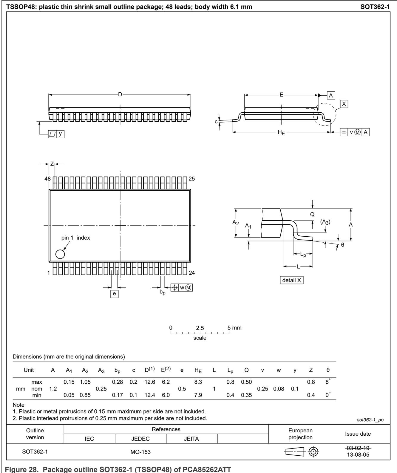
Figure 28. Package outline SOT362-1 (TSSOP48) of PCA85262ATT
