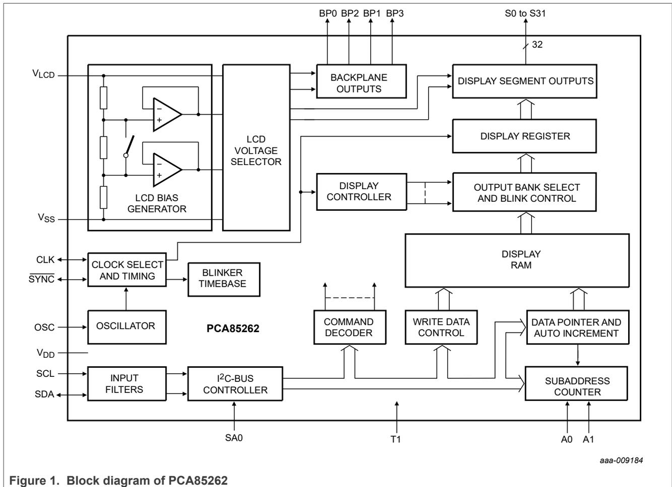
Figure 1. Block diagram of PCA85262
