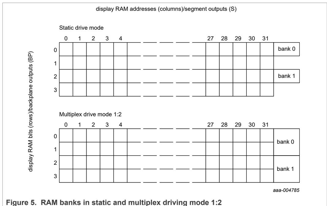
There are two banks; bank 0 and bank 1. [Figure 5](#) shows the location of these banks relative to the RAM map. Input and output banks can be set independently from one another with the Bank-select command (see [Table 9](#)). [Figure 6](#) shows the concept.
