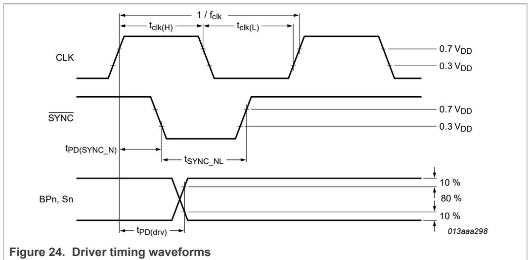
Figure 24. Driver timing waveforms
