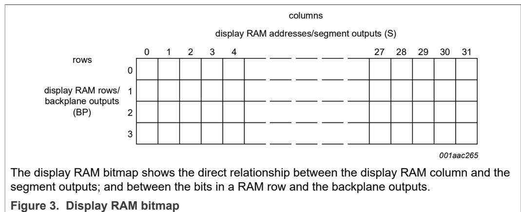
When display data is transmitted to the PCA85262, the display bytes received are stored in the display RAM in accordance with the selected LCD drive mode. The data is stored as it arrives and depending on the current multiplex drive mode the bits are stored singularly, in pairs, triples or quadruples. To illustrate the filling order, an example of a 7-
