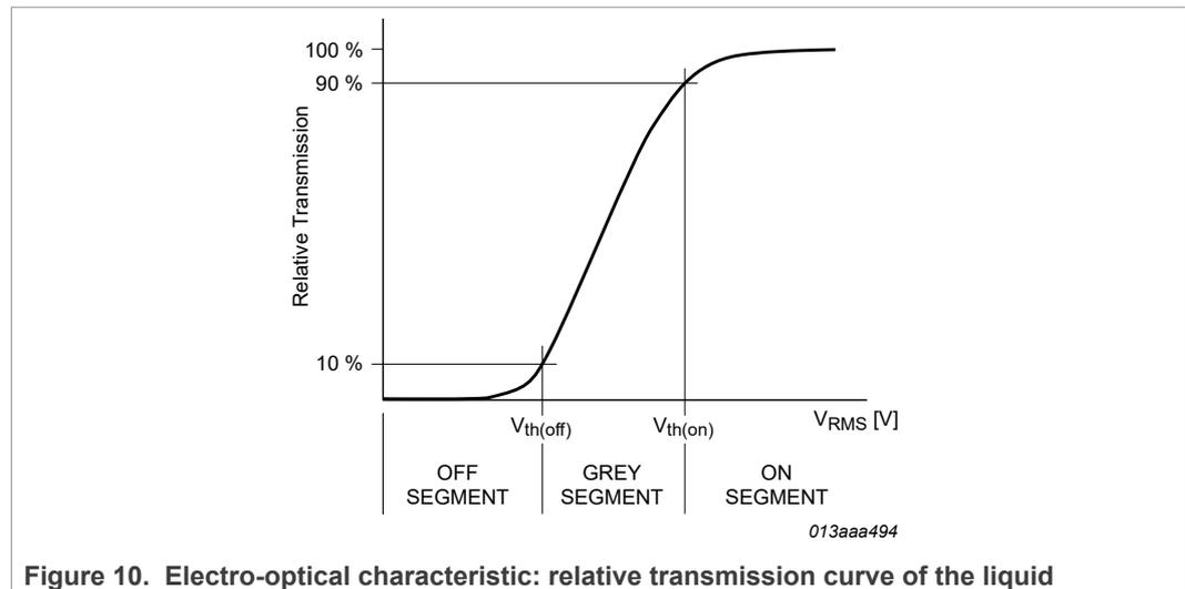
Figure 10. Electro-optical characteristic: relative transmission curve of the liquid
