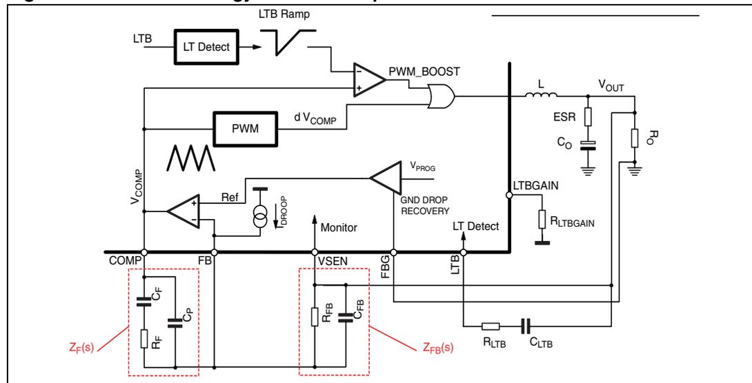
The LTB detector is able to detect output load transients by coupling the output voltage through an R<sub>LTB</sub> - C<sub>LTB</sub> network. After detecting a load transient, the LTB ramp is reset and then compared with the COMP pin level. The resulting duty-cycle programmed is then OR-ed with the PWM signal by-passing the main control loop. The phase will then be turned-on and the EA latencies results bypassed as well.
