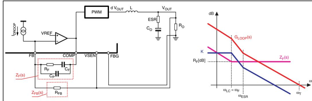
To obtain the desired shape an  $R_F - C_F$  series network is considered for the  $Z_F(s)$  implementation. A zero at  $\omega_F = 1/R_F C_F$  is then introduced together with an integrator. This integrator minimizes the static error while placing the zero  $\omega_F$  in correspondence with the L-C resonance assures a simple -20 dB/dec shape of the gain.
