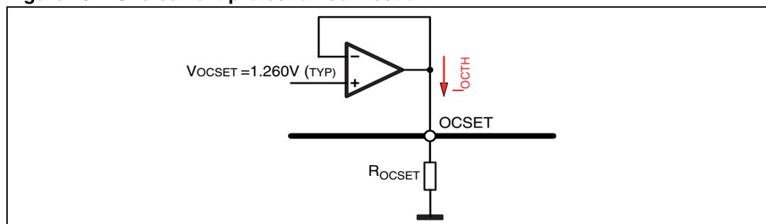
**Note:** In order to avoid the OCP intervention during the DVID, the device automatically increases the OCP threshold to 150% of the selected OCP threshold during every VID transition (adding an extra 15  $\mu$ s of delay).
