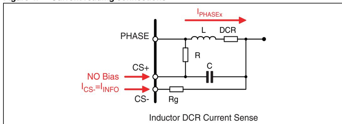
Considering now to match the time constant between the inductor and the R-C filter applied (Time constant mismatches cause the introduction of poles into the current reading network
