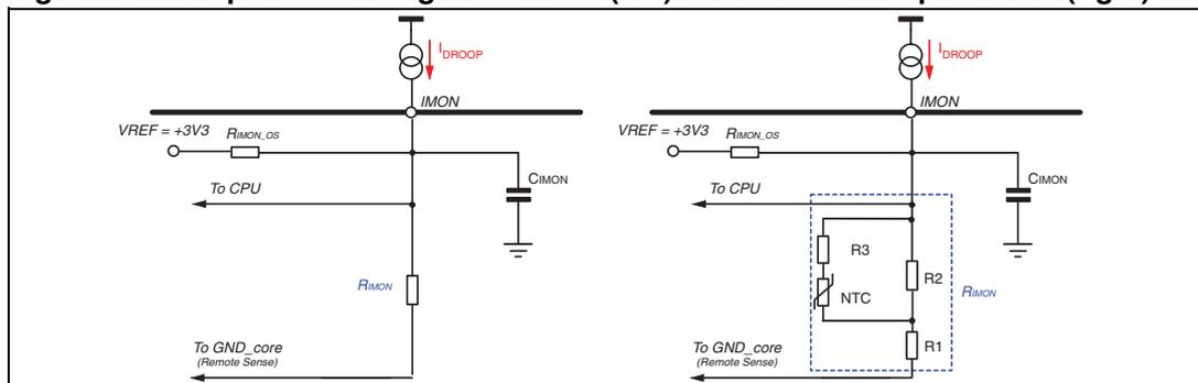
Current sense element (DCR inductor) has a non-negligible temperature variation. As a consequence, the sensed current is subjected to a measurement error that causes the monitoring voltage to vary accordingly.
