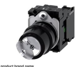
RONIS key-operated switch, 22 mm, round, plastic, lock number SB30, with 2 keys, 2 switch positions O-I, latching, 10:30h/13:30h, key removal O+I, with holder, 1 NO, screw terminal, possible special locks: SB31, 421, 455
